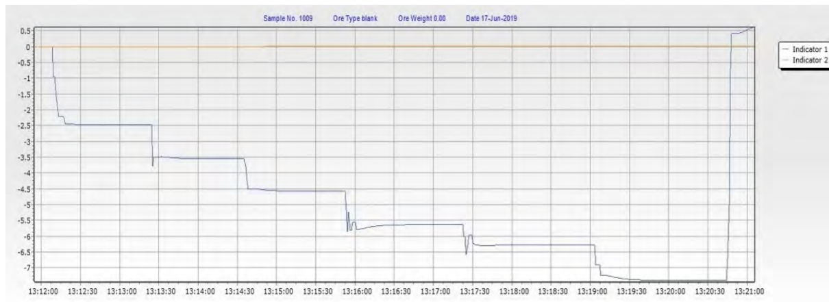
Graph 10. Blank, no ore friction trace at selected speeds of 1.5, 1.75, 2.0, 2.5, 3.0 and 3.5 m/s.
