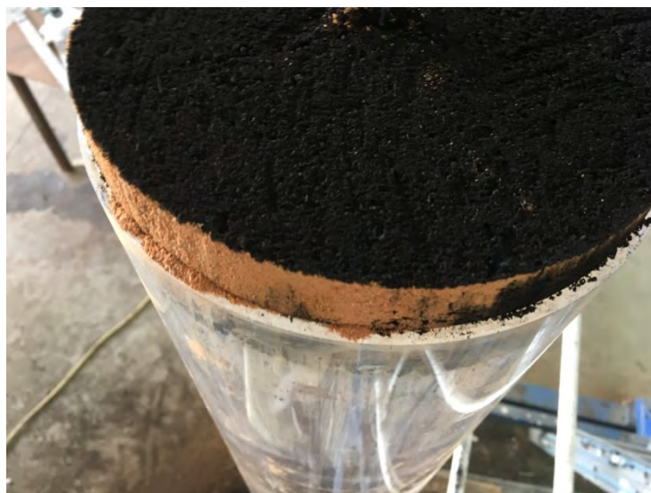
Picture 28. Coal under gravel after 1500mm movement with the upper layer of gravel removed.
