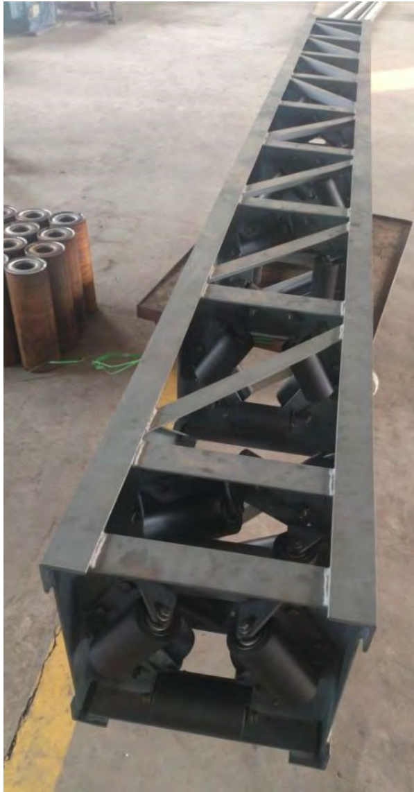
Picture 3K Pipe conveyor section without the conveyor belt fitted
