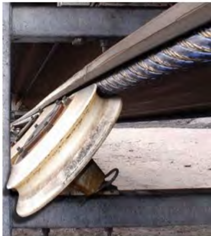
Picture 1 Cable belt. Metso MRC Cable belt conveyor (Metso, 2019).
