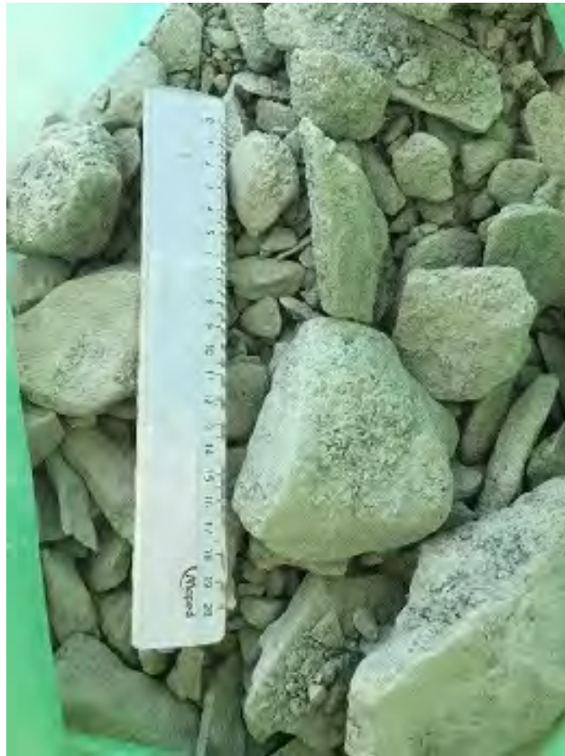
Picture 8. Ungraded granite after blasting.
