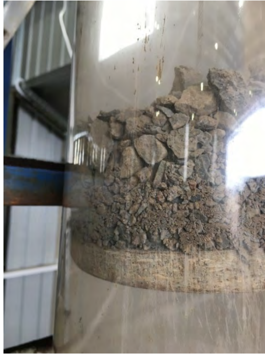
Picture 33. Ungraded granite after 1000mm of movement.
