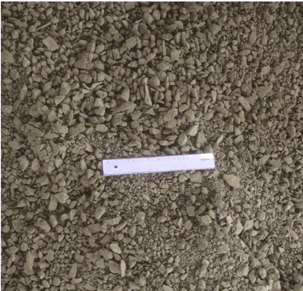
Picture 46. Crushed ungraded granite.
