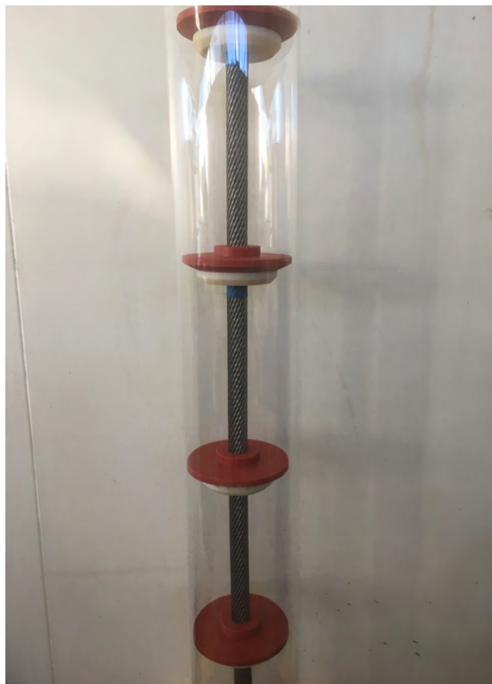
Figure 5: The cable disc elevator sketch as in figure 2 and a clear view of the cable disc elevator section in a plastic tube.
