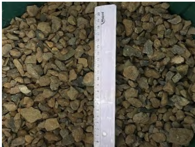
Picture 9. Crushed Granite over 9.5mm.
