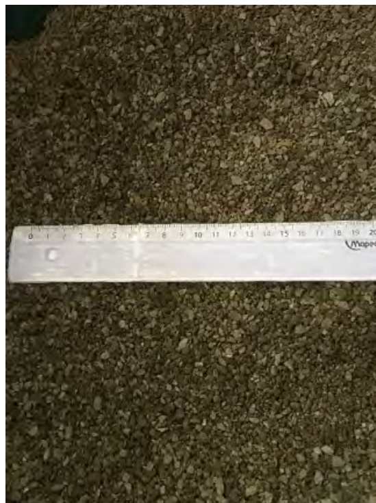
Picture 11. Crushed Granite over 2mm less than 5mm.
