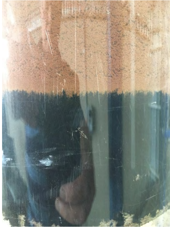
Picture 21. Coal under gravel after 250mm of movement.
