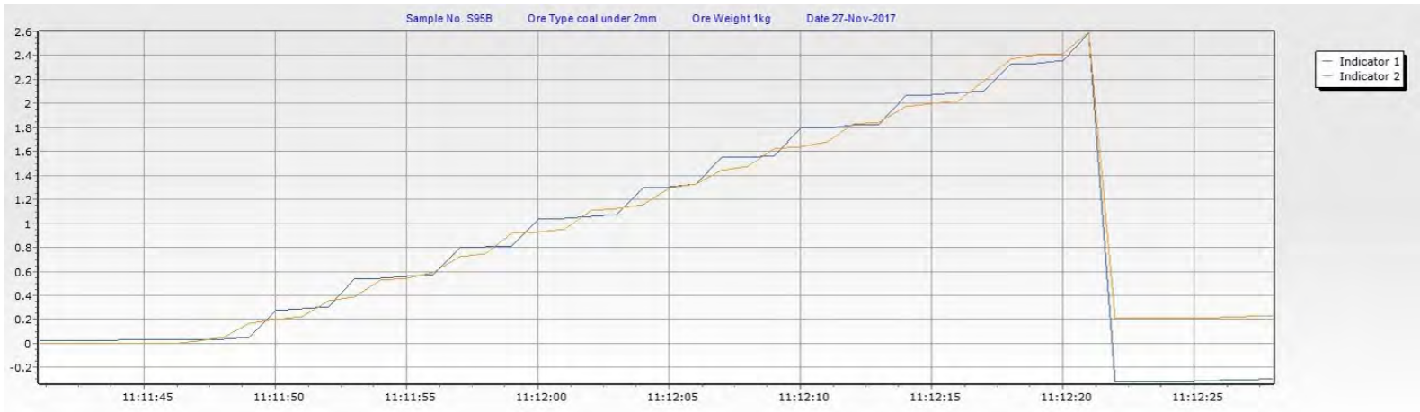
Graph 3. Coal 2mm particle size. Breakfree force test 1000g. Water is added to the bucket at 2litres per minute
