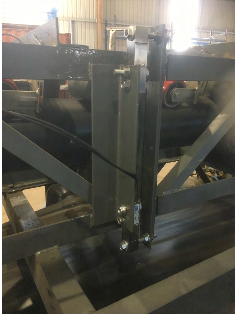
Picture 3B. Test rig 3 pipe conveyor 6 roller centre panel mounted on load cells
