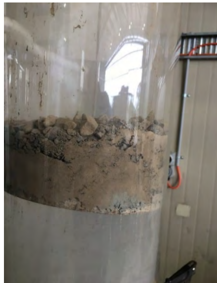
Picture 30. Ungraded Granite after 250mm of movement.
