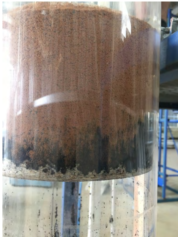
Picture 26. Coal under gravel after 1500mm of movement.
