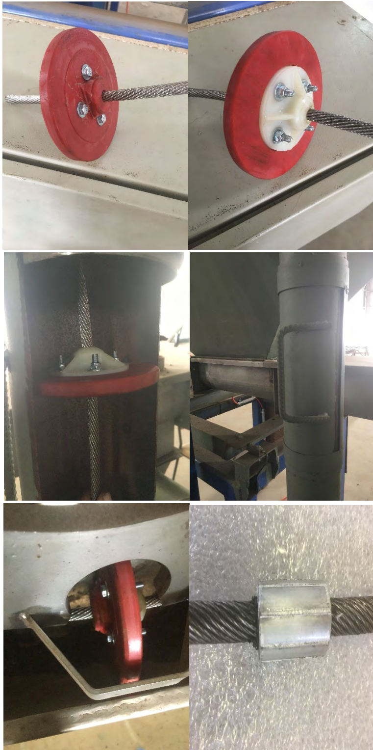
Picture 2F. Test Rig 2 Elevator disc segments mounted on the Crosby cable swages
