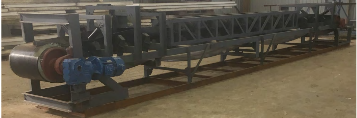
Picture 49. Test Rig 3. This shows all sections including section 4, which is the return of the belt to the lower idle roller under the pipe conveyor.
