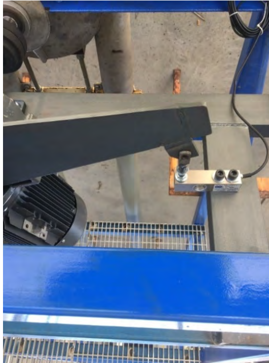
Picture 2C. Test Rig 2 torque arm and load cell
