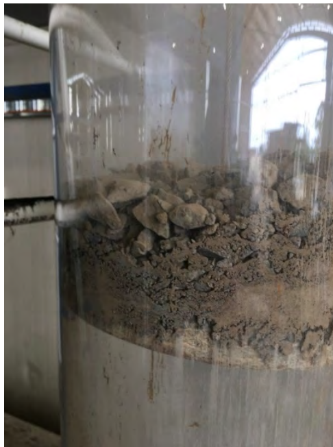
Picture 32. Ungraded granite after 750mm of movement.
