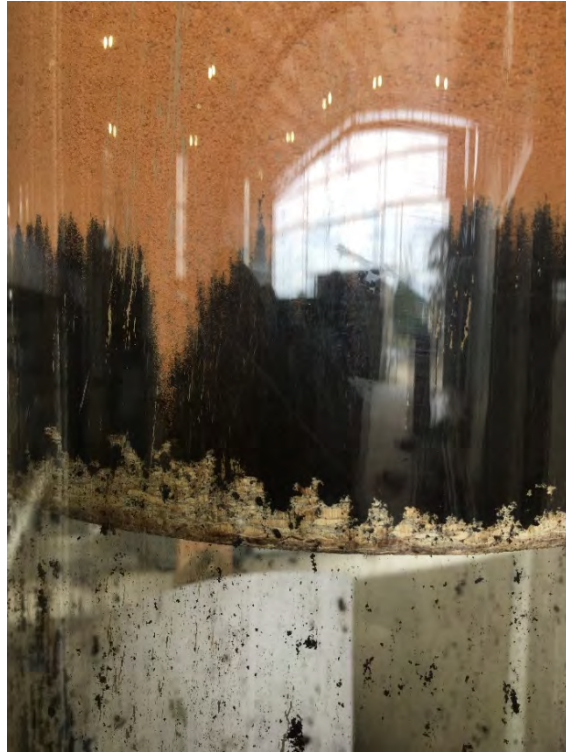
Picture 23. Coal under gravel after 750mm of movement.
