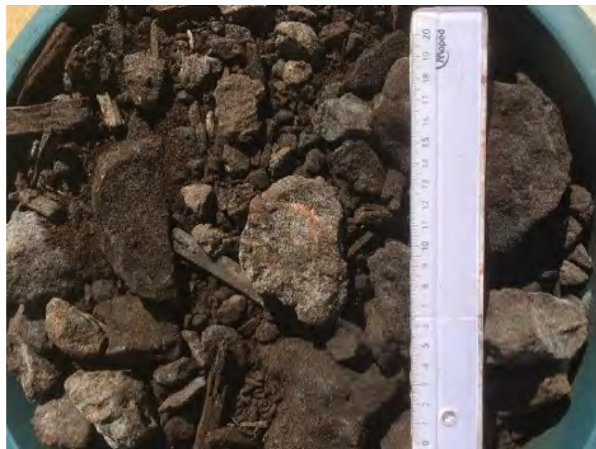
Picture 4. Ungraded Coal prior to the crushing plant.
