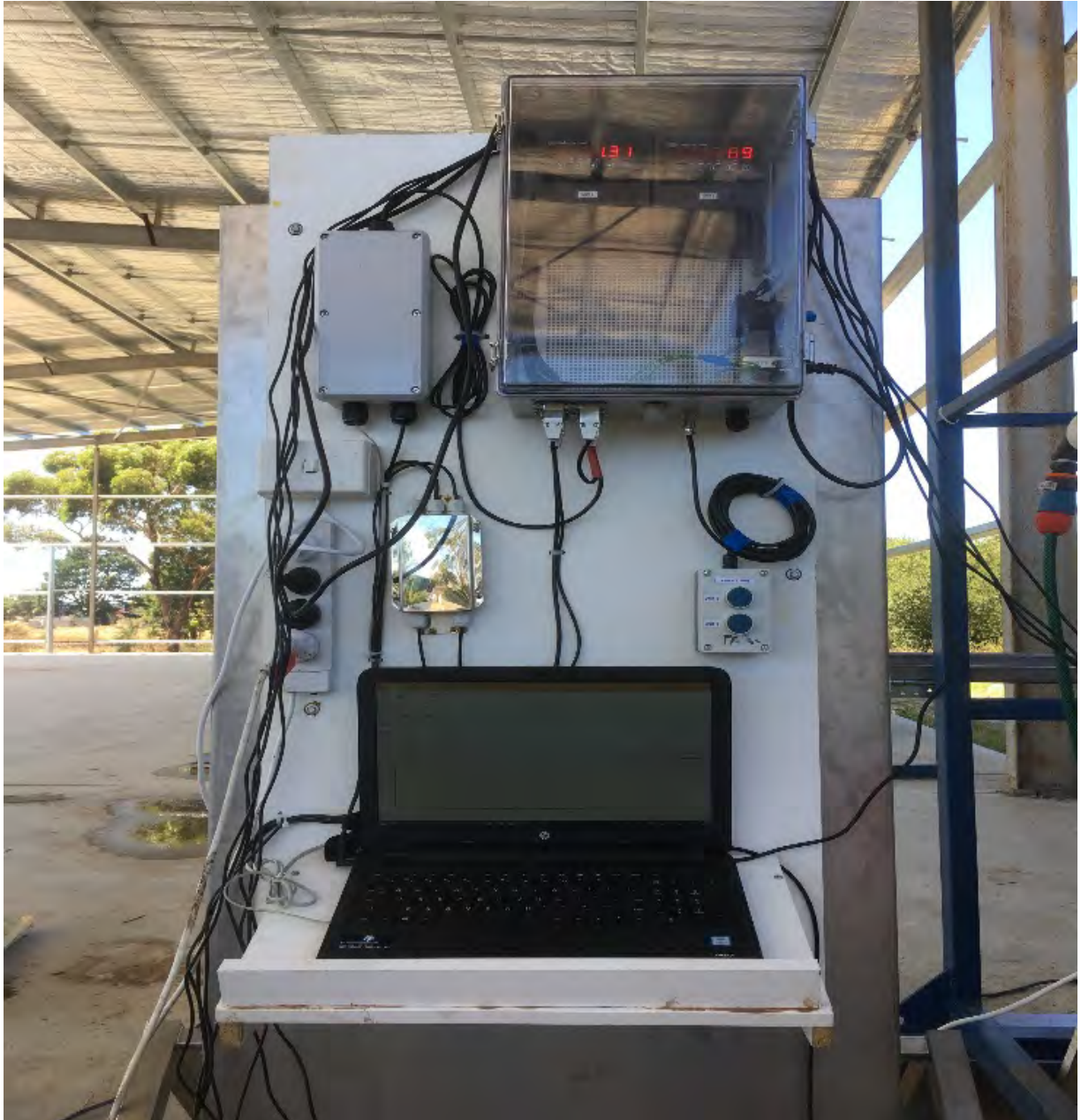
Picture 1A. Test Rig 1 Instrumentation showing the load cell weights, two tare buttons, and computer with software programming.
