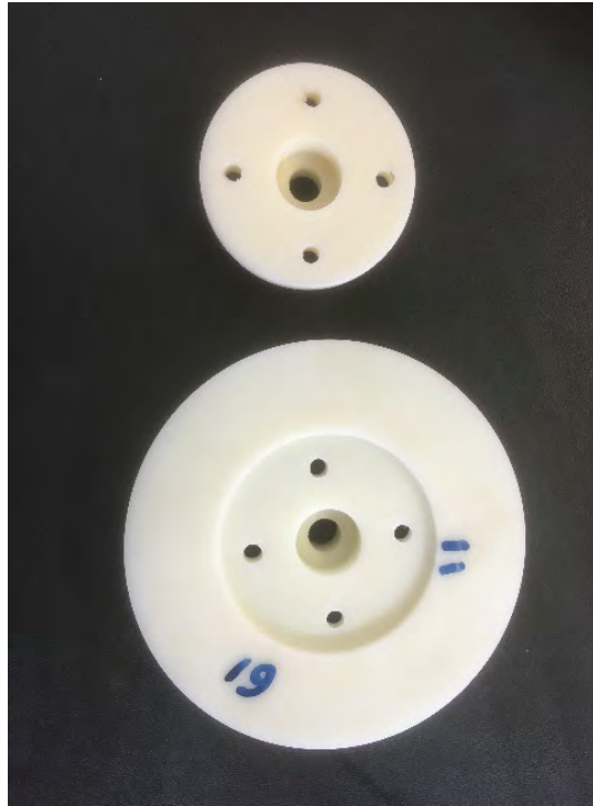
Picture 3F Cable elevator discs joining side
