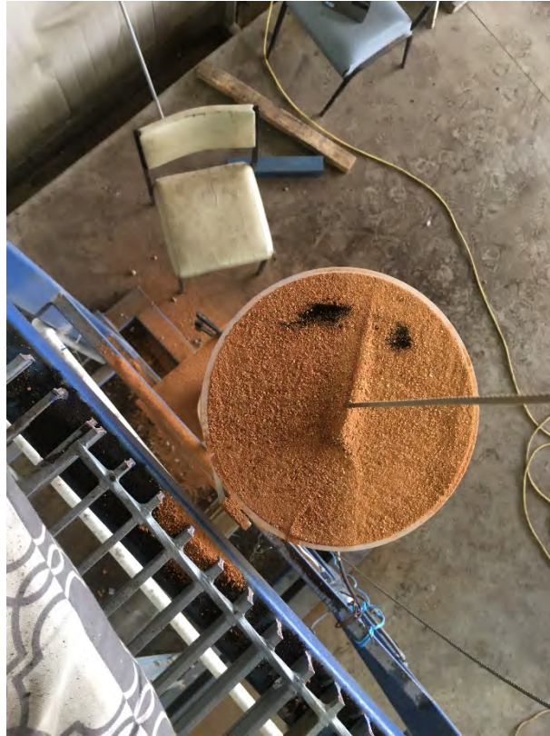
Picture 27. Coal under gravel after 1500mm movement. Top View.
