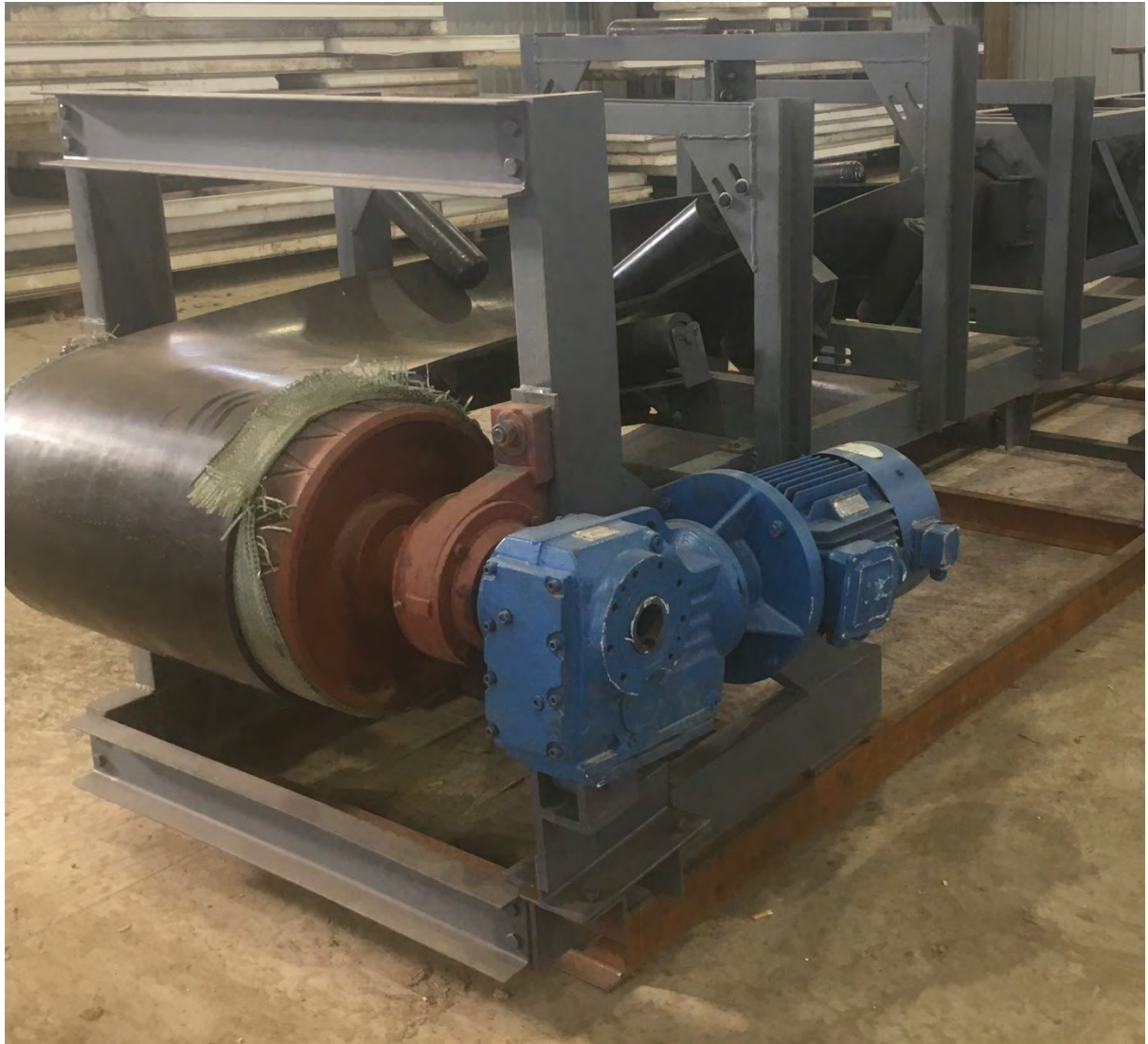
Picture 3L. Pipe conveyor drive end
