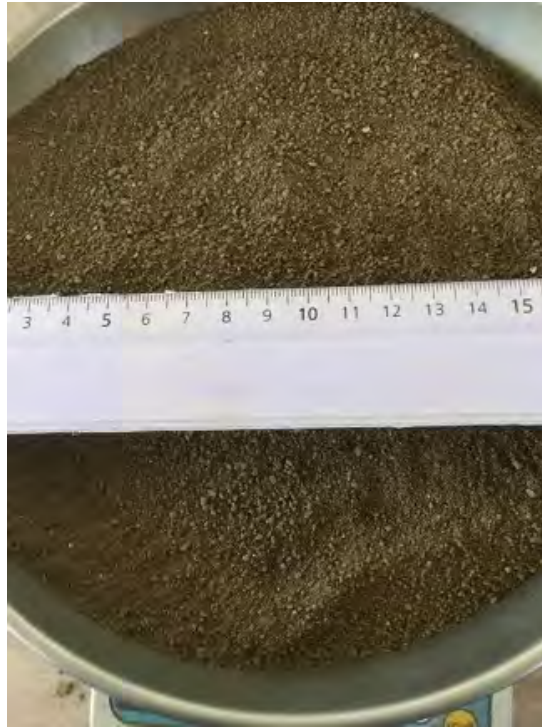
Picture 12. Crushed granite less than 2mm.
