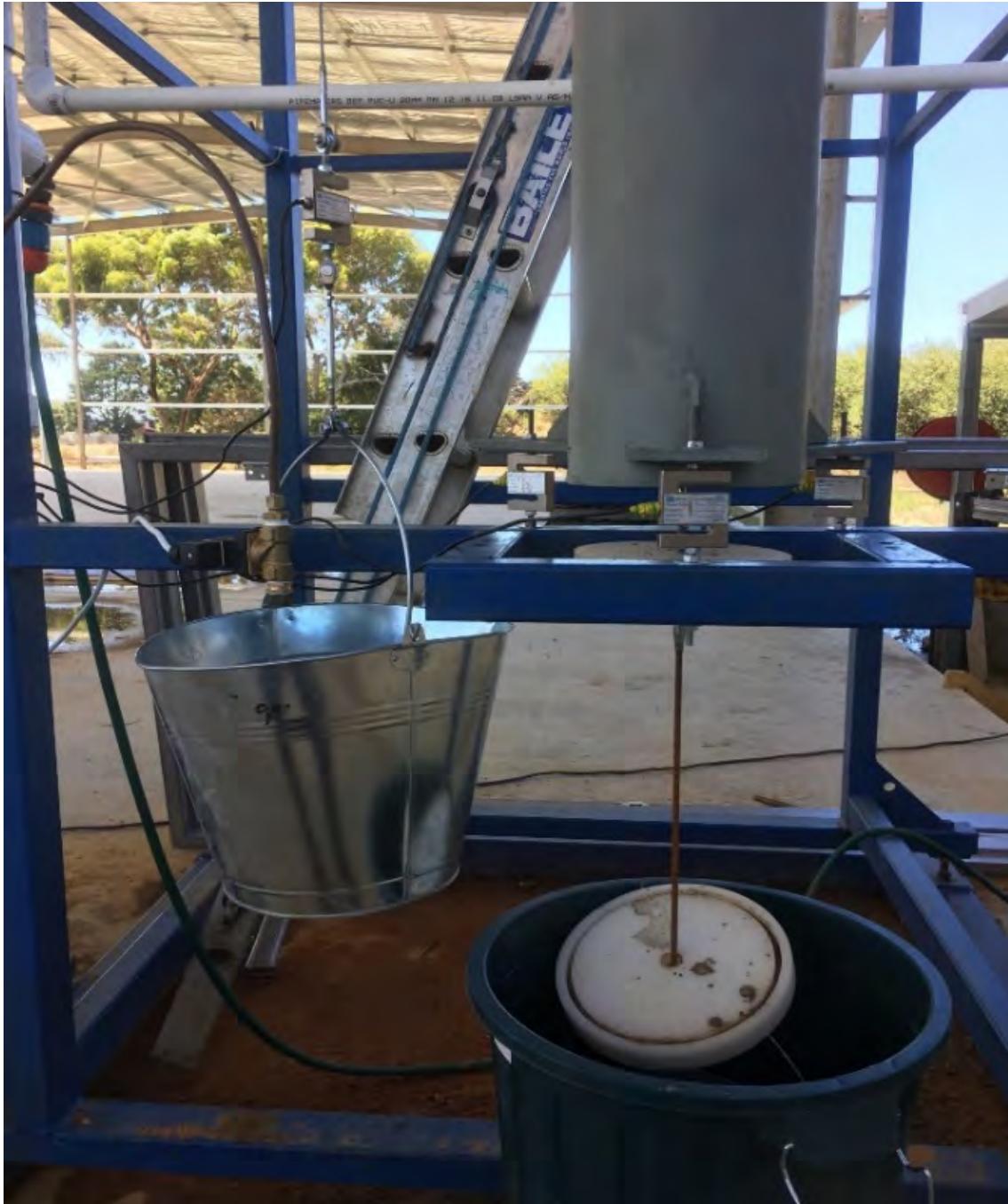
Picture 1C. Test Rig 1 lower section in more detail. The counterweight bucket hanging on a ‘S’ shape load cell, tube base plate, the lifting disc is just under the ore tube that is mounted on 3 ‘S’ shape load cells. The water discharge solenoid valve is just above the bucket.
