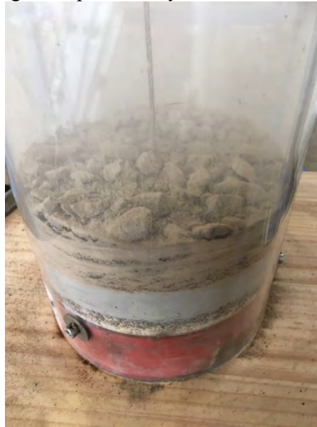
Picture 29. Ungraded granite at zero movement.
