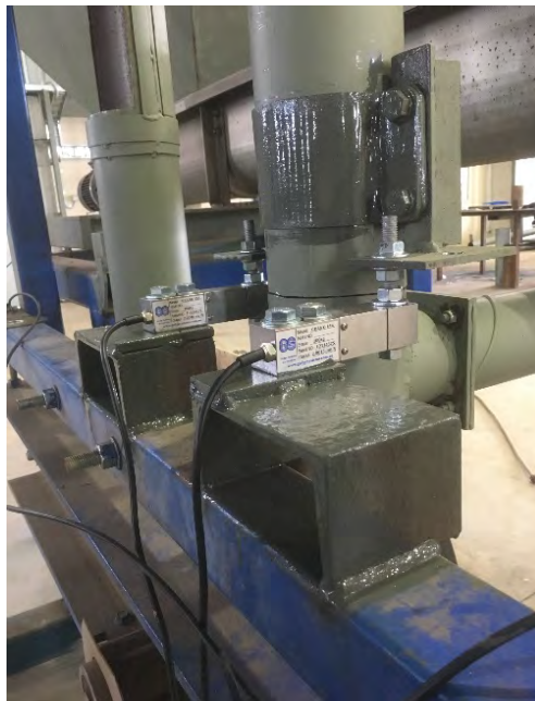
Picture 2B. Test Rig 2 showing the lower 2 of the 4 load cells that the lifting tube is mounted on.
