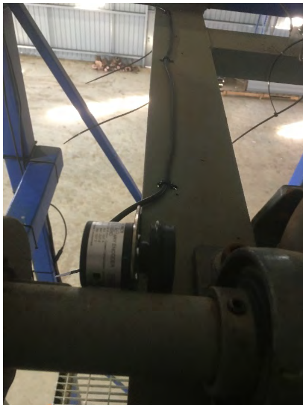
Picture 2D. Test rig 2 drive shaft RPM encoder for shaft speed.
