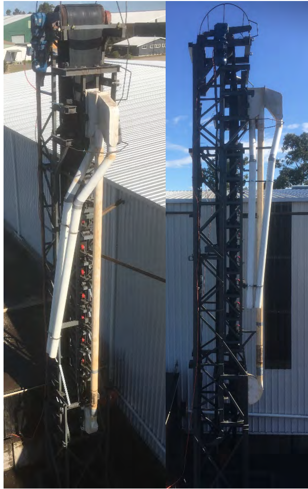
Picture 42. Front and side view of Test Rig 2 without the ore bin
