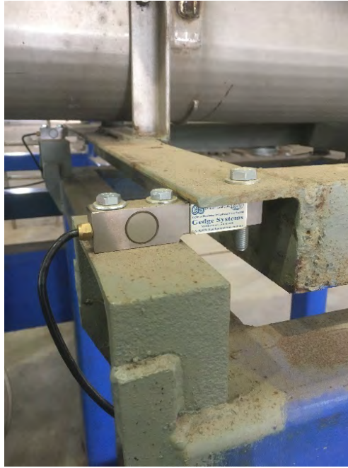
Picture 2A. Test Rig 2 ore bin mounted on 4 load cells, one of the load cells is in the foreground
