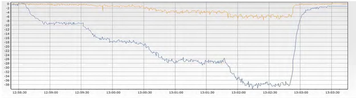
Graph 18. 2mm Granite. Elevator speed 3.0 metres per second. Ore bin speed 11, 22, 33, and 44. Data from Appendix 3, Table 204.
