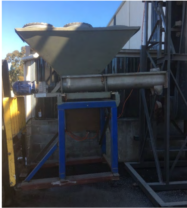
Picture 45. The ore bin.
