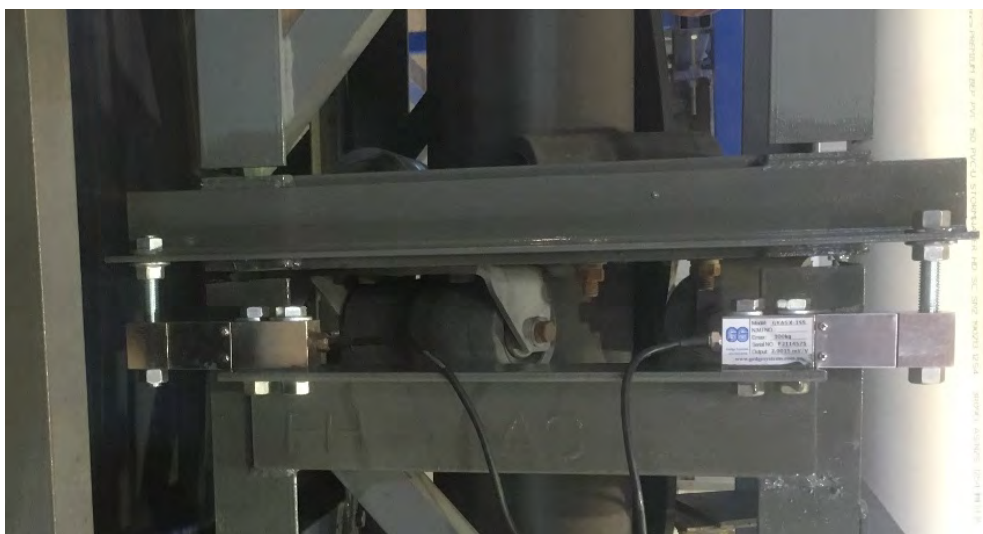
Picture 3C. Test rig 3 pipe conveyor centre panel 2 of 4 load cells
