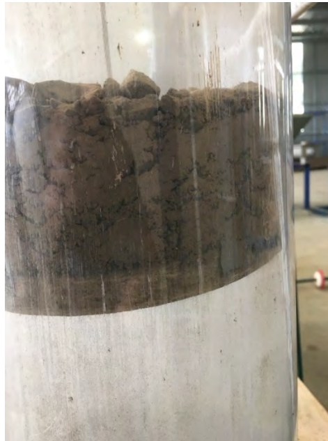
Picture 31. Ungraded Granite after 500mm of movement.
