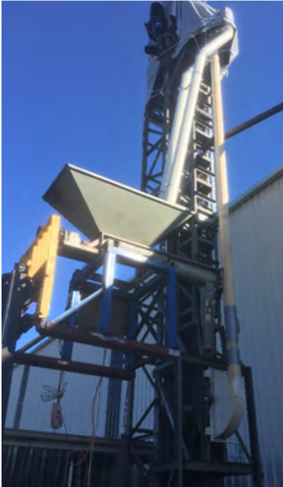
Picture 3E. The hybrid elevator. Weather cover on top and the ore bin in position for operating. The ore bin was lifted up for operation and lowered to ground level for emptying and changing the ore.
