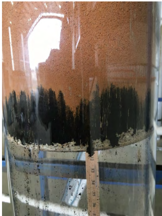
Picture 24. Coal under gravel after 1000mm of movement.
