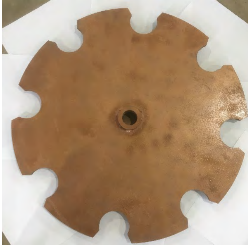
Picture 43. Cable sheave with 8-disc slots, used for the drive and idle sheaves.
