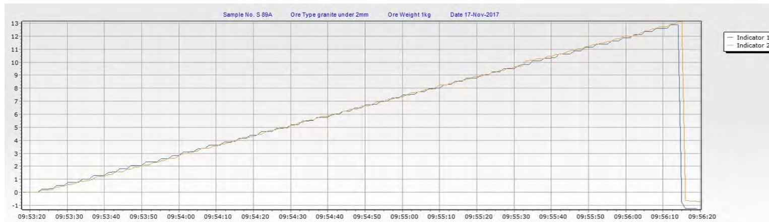
Graph 2. Granite 2mm particle size. Breakfree force test 1000g. Water is added to the bucket at 2litres per minute
