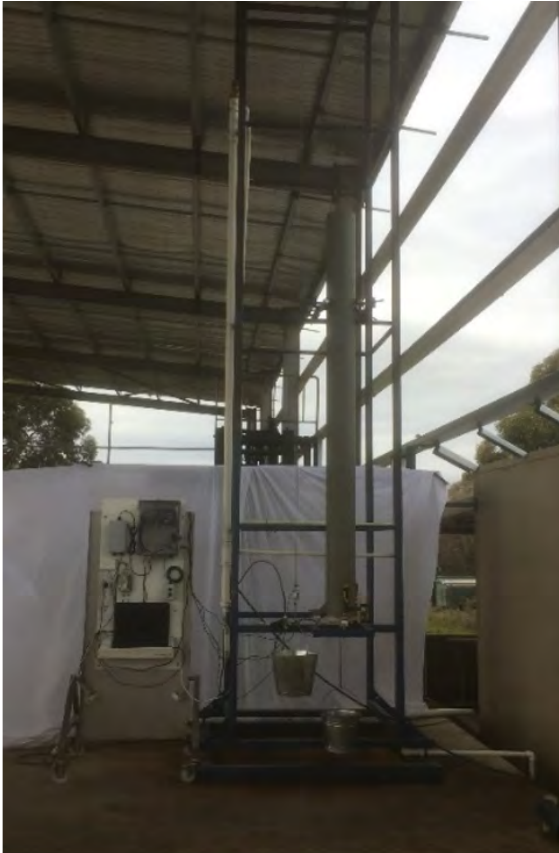
Picture 1B. Full test rig showing the instrument and control panel, counter weight bucket hanging on a load cell, the test ore tube mounted on 3 load cells, and the white pipe part of the constant head water flow system that discharged through the solenoid valve.
