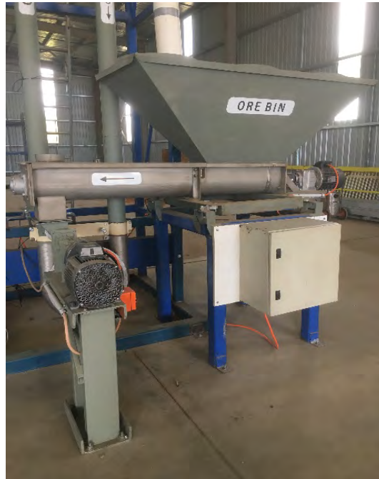
Picture 41. Ore bin mounted on 4 load cells.
