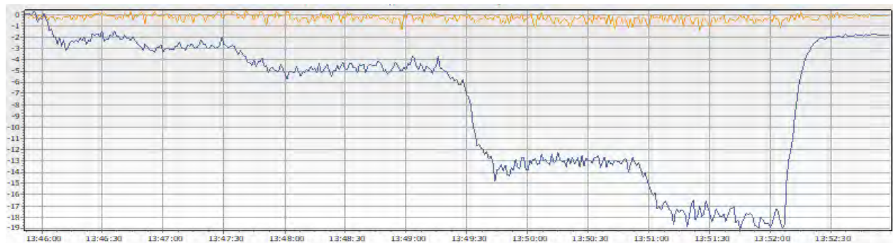
Graph 22 Coal 2mm ore size. Ore feed constant elevator speed at 3.0 m/s. Ore bin speed increased in steps. 11,22,33 and 44 RPM. Appendix 3 Table 210.
