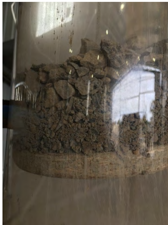
Picture 34. Ungraded granite after 1250 mm of movement.
