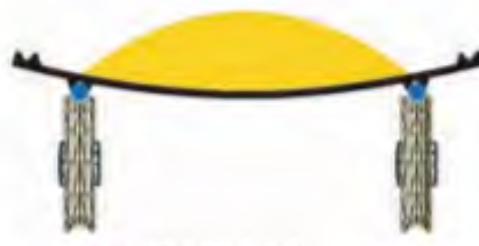
Picture 1 Cable belt. Metso MRC Cable belt conveyor (Metso, 2019).
