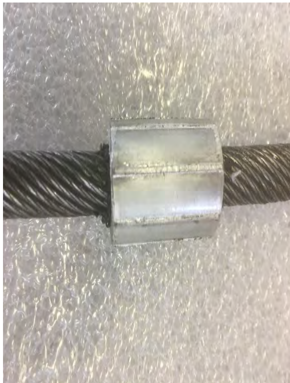
Picture 3I. Crosby swage on the cable disc elevator cable
