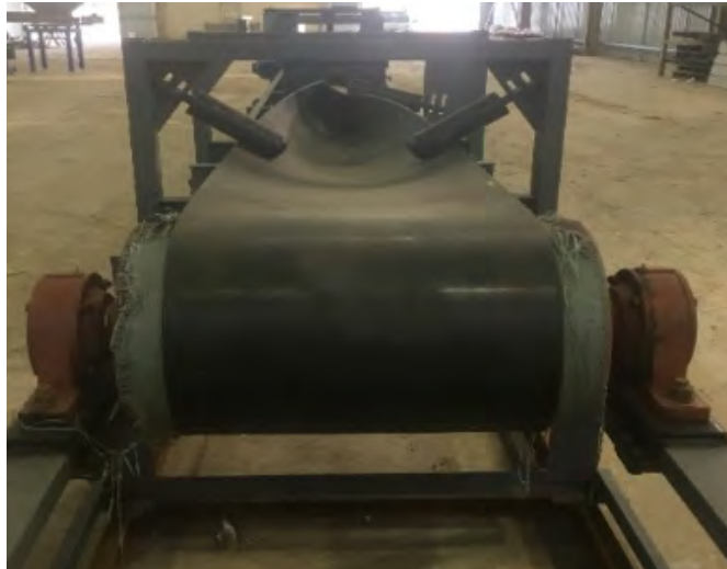
Picture 48. Test rig 3. Pipe conveyor, tube forming end section 1.
