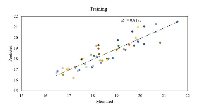
Figure 3 The proposed MR model to estimate rock cohesion
