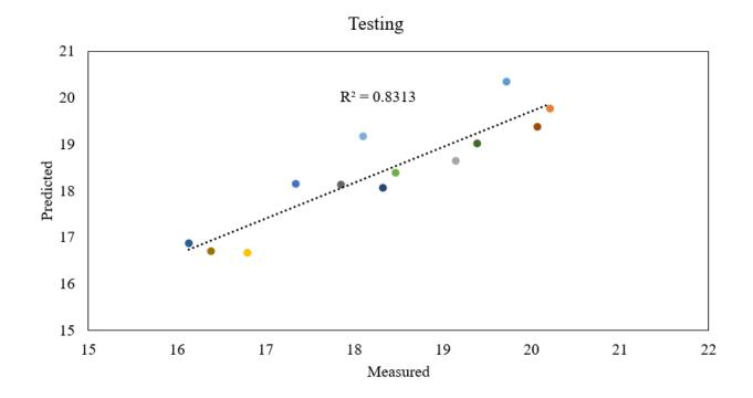
Figure 4 The proposed MR model to estimate rock cohesion
