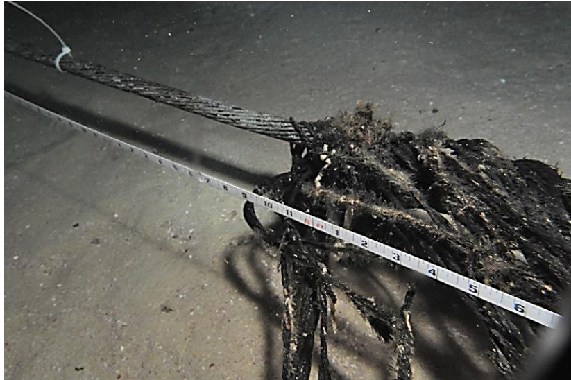
Figure 13: Outer sheathing damage and armour exposure due to instability
