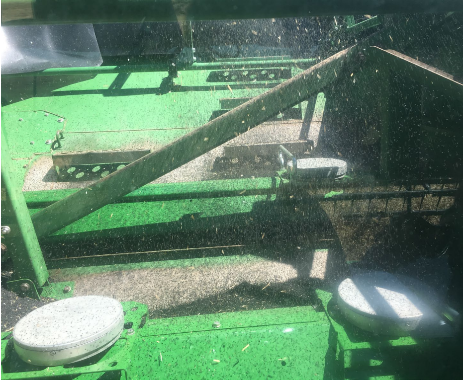
Figure 11. A photograph of the grain tank filling with canola, taken from the header cabin through the rear window.
