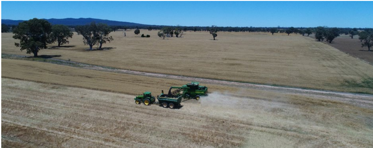
Figure 31. This photograph captures the header auger extended over the chaser bin and unloading the canola while in transit. One person is in each cabin operating the machine. The drain was previously cut by an excavator to shed paddock water, and it divides the paddock of canola from the paddock of wheat.
