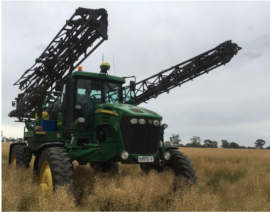
Figure 7. The undercarriage of the self-propelled sprayer was equal height to the hybrid canola.
