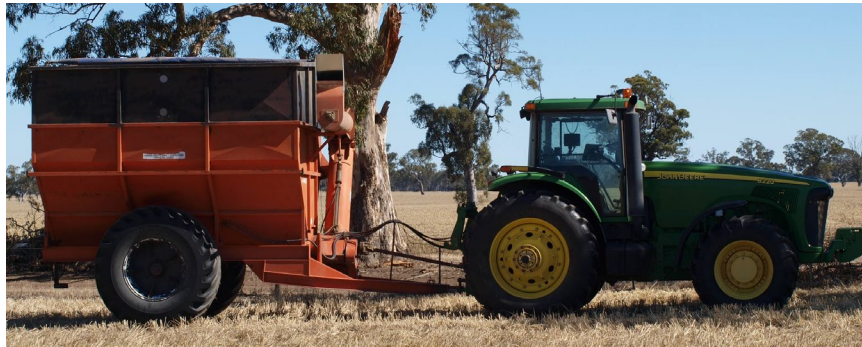
Figure 21. The photograph shows the chaser-bin extension in a contrasting colour to its factory-made size.
