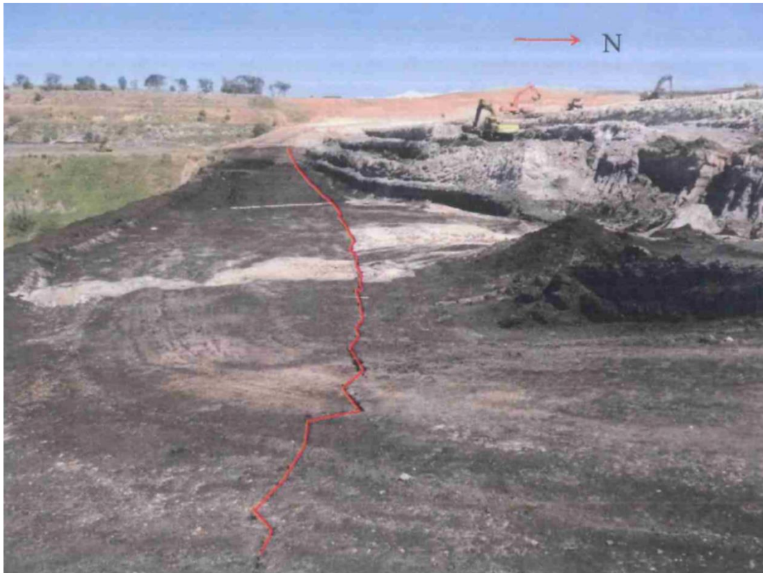
Figure 4.2 Crack on the coal seam (looking towards west)
