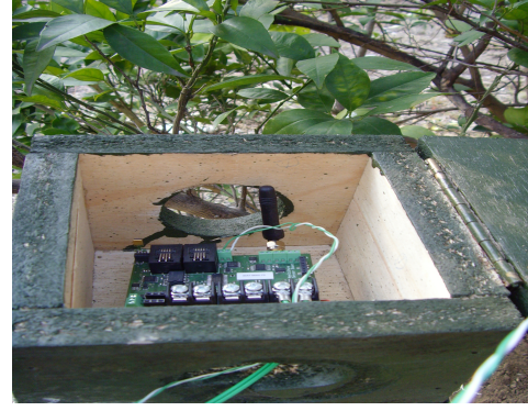
Fig. 1. Deployment of the Wasp-Mote Agriculture Boards with Humidity and Temperature Sensors
