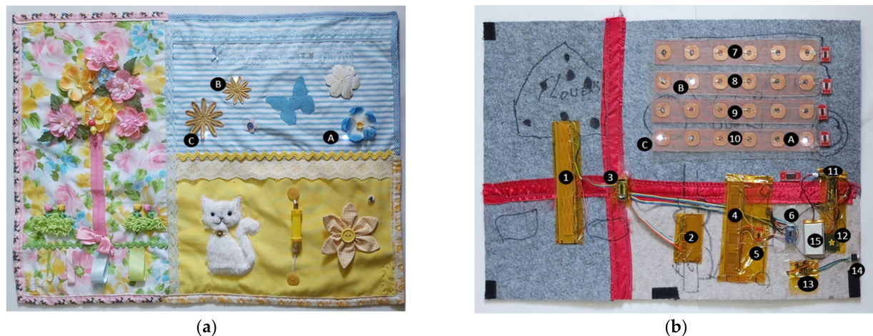
Figure 3. The two layers of the smart textile: (a) textile layer with persona metaphors—including cat, tree, sky; (b) technological layer where all the components are attached (refer to Table 1 for the list of components).
