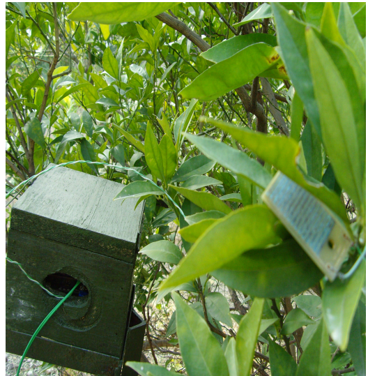
FIGURE 4. Leaf wetness sensor deployment near plant leaves.
