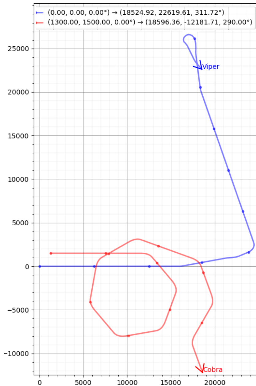
Figure 4.8: The trajectory of ac-005 for complex scenario 2. Distances are in metres
