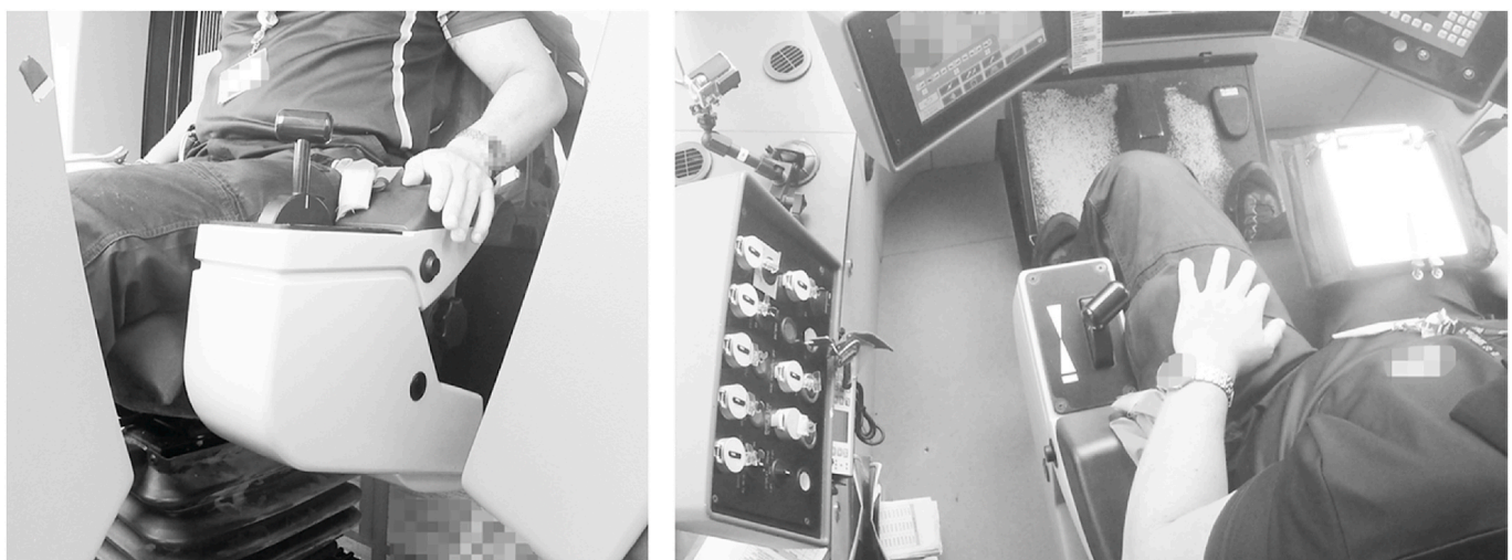
Fig. 4. View inside the driver-cab as observed through cameras mounted on the console facing the driver from the side (left photo), and down the driver's body from the top (right photo). A side-mounted camera can be viewed in the top camera view. Note the radio button built into the footpedal in the right photo.
