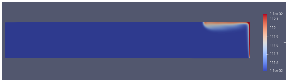
Figure S2.1: Vapour temperature profile in the CFD simulation of the isobaric evaporation of methane for the test case, Scenario 1 ( V_T = 8\text{m}^3 , LF = 0.97 ), after 10 seconds of simulation.
