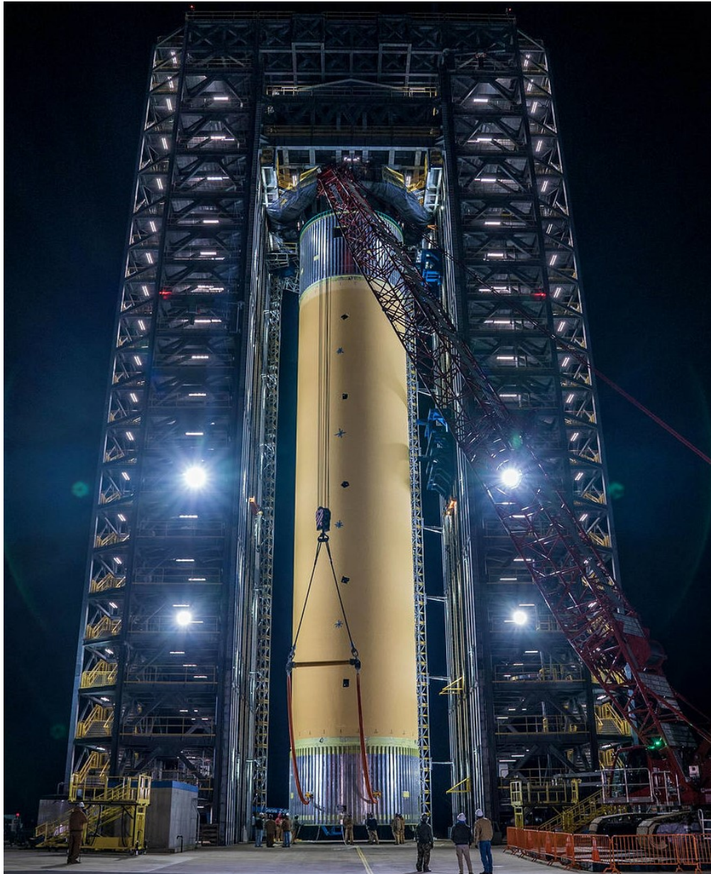
Figure 1.2: NASA 2,033 m 3 liquid hydrogen tank. This tank is a part of the space launch system (SLS) in the Marshall Space Flight Center in Huntsville, Alabama, U.S.A. Reprinted from NASA, 2019, from: https://www.nasa.gov/exploration/systems/sls/nasa-engineers-break-sls-test-tank-on-purpose-to-test-extreme-limits.html
