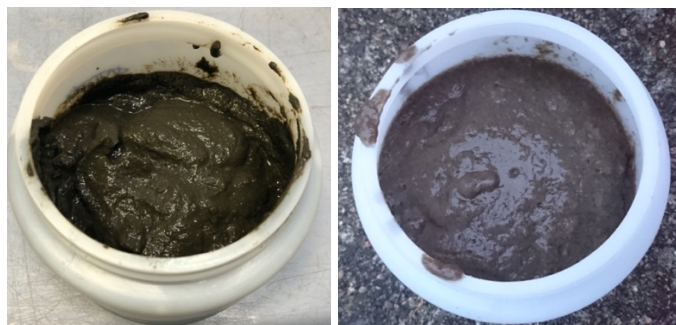
Figure 3-4 (a) Wasted activated sludge sample from sludge thickening belt; (b) mixed liquor sample from aerated tank
