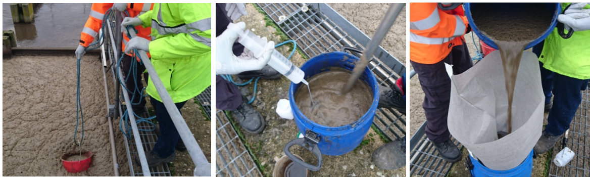
Figure 3-3 Sampling mixed liquor and dosing Flopam on-site
