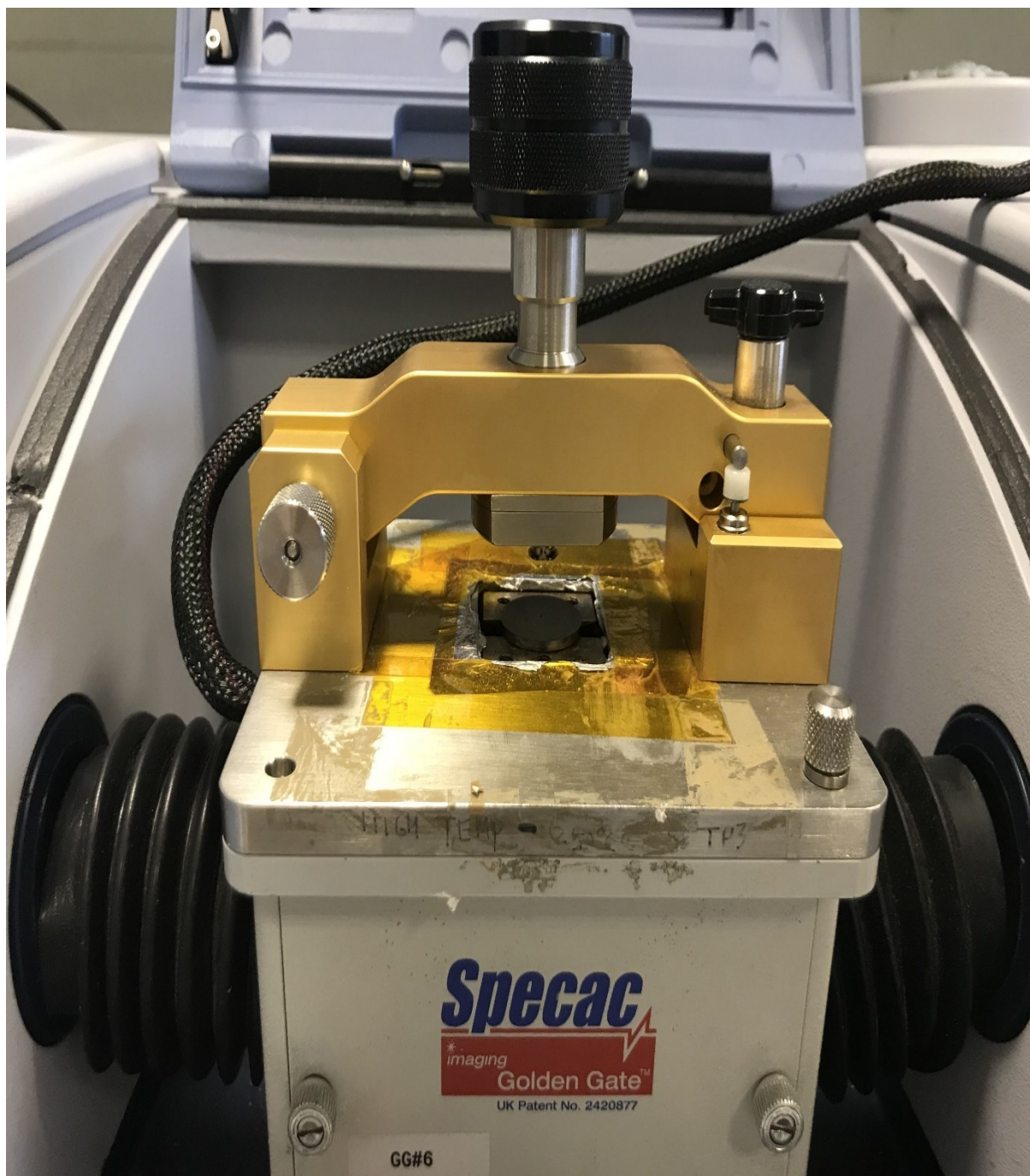
Figure 3.13 Photograph of the Imaging Golden Gate™ ATR accessory in the IMAC macrochamber.
