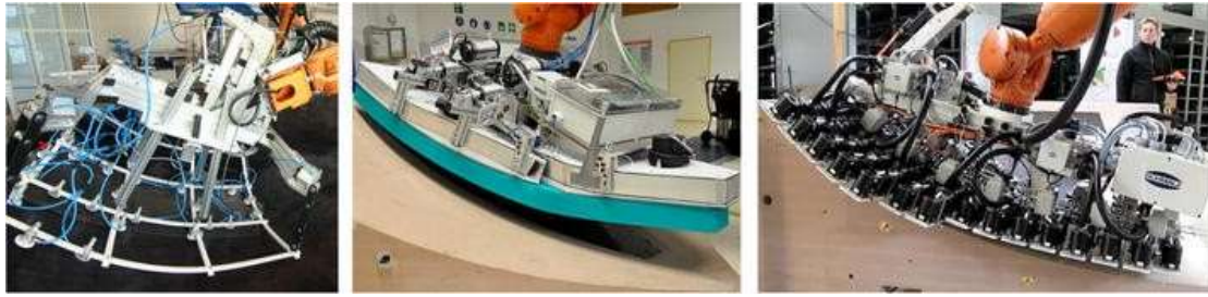
Figure 3.7: A second example of a robotic end effector gripping and draping system with integrated heating cells. This example highlights a much larger end effector array and the double curvature target geometry [54].
