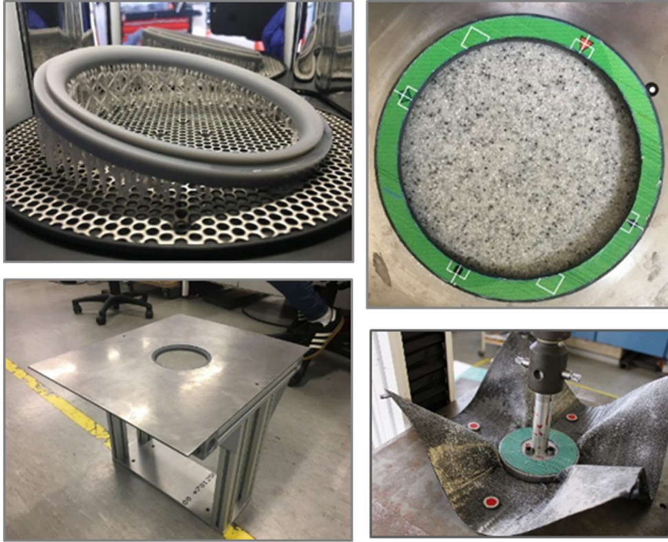
Figure 6.3: (Top-left) The hemisphere radial insert after curing showing recess bond line, (top-right) the reverse of the insert showing the calibration markings, (bottom-left) subsequent insertion to the forming bed, (bottom-right) example forming operation.
