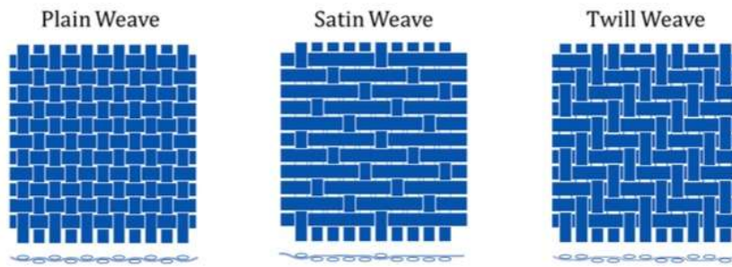
Figure 2.2: Examples of three major weave patterns with the corresponding degree of crimp highlighted [11].
