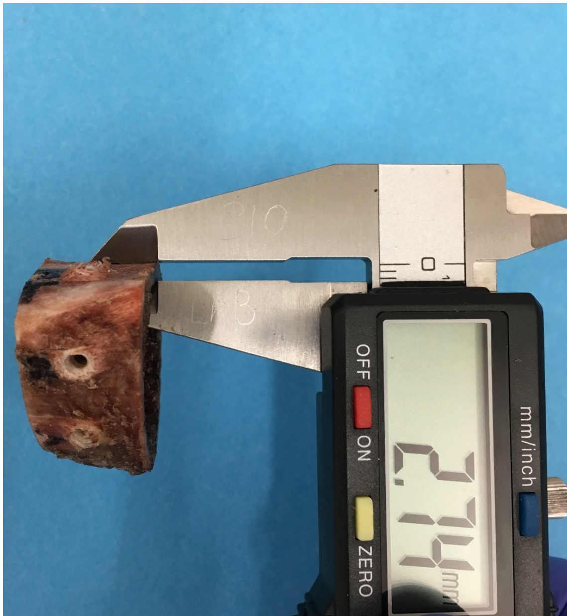
Figure 3-4 - Measuring cortical thickness of juvenile bovine sample.
