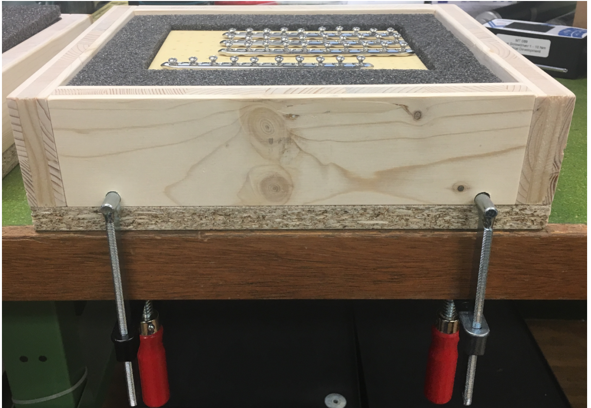
Figure 6-2 - Testing apparatus – screw drill holes made following 10-hole, 3.5 mm LC-DCP template, with artificial bone sheet placed into dense foam, on top of a less dense foam – the latter mimicking the stiffness of human tissue.
