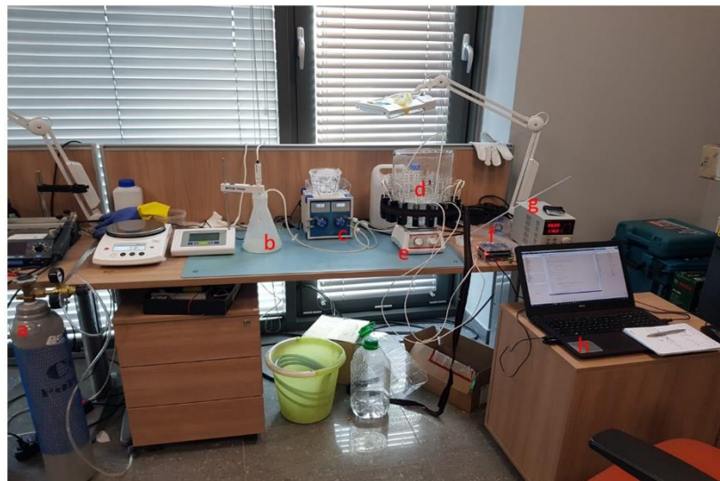
Figure 5.7. Photo of the batch crystallization experimental apparatus. (a) Carbon dioxide tube for gas injection, (b) reagent vessel filled with sodium carbonate solution (reagent), (c) electronic peristaltic pump, (d) receiving tank filled with calcium chloride solution, (e) IKA Midi 1 digital magnetic stirrer, (f) tomographic device developed by NETRIX company, (g) power supply, (h) computer unit used for running MATLAB code and providing tomographic results.
