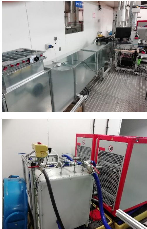
Figure 3-7: Wind tunnel and the Cooling circuit, respectively
