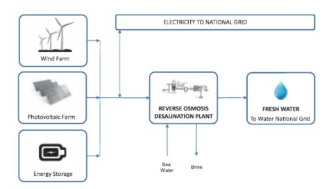
Figure 15. Process Diagram for Monsson Target Project [82]
