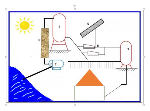
Figure 16. Design of the PV-RO Desalination Unit
