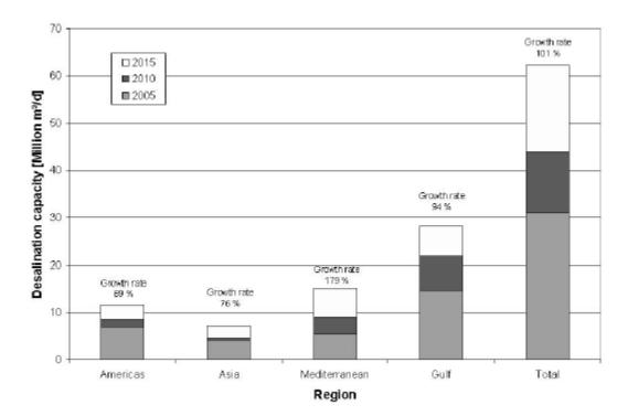
Figure 3. Expected Growth in Desalination Capacities [5]
