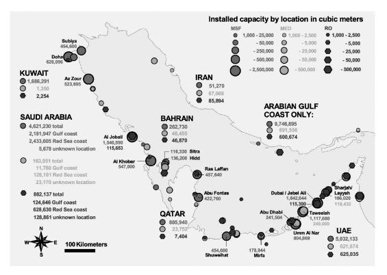
Figure 2. Seawater Desalination in the Arabian Gulf [4]
