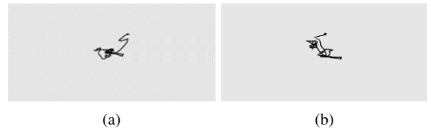
Fig. 15: Gmapping trajectory in long corridor: (a) Walking mode 1: standard speed, smooth rotation. (b) Walking mode 2: fast speed, sharp rotation.
