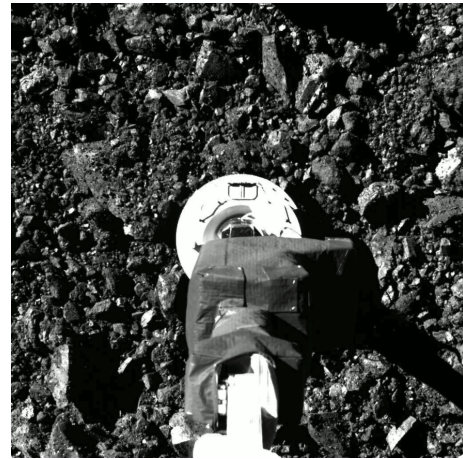
(B) IMAGE CAPTURED DURING THE OSIRIS-REX TOUCH-AND-GO SAMPLE COLLECTION EVENT OF BENNU, JUST BEFORE TOUCHDOWN. 7
