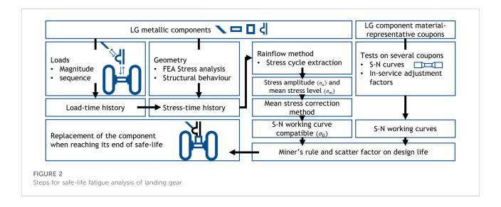
accumulated from the stress formed by the cycles. As (Hoole, 2020) mentions, a value of 1 for  $(D_T)$  signifies failure of the part in question, meaning it has reached the end of its fatigue life, and representing failure Eq. 3.
