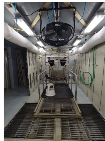
Figure 1. Schematic view and overview photo of the climate-controlled respiration chamber. There are 2 temperature sensors hanging on each side wall (left and right), and 1 temperature sensor and 1 relative humidity sensor hanging on the wall in front of the cow. The material of the solid floor is rubber mat, and the slatted floor is rubber-covered metal grills (Gerrits and Labussière, 2015). The cow inside the chamber was tied up loosely so that it could easily move forward or backward and lie down.
