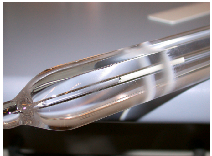
Fig. 1. Preform prepared for drawing (rod-in-tube method) with silica rod for drawing process start-up phase followed by Tm:YAG crystal.
