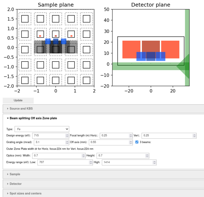
Fig. 3. BOZ calculator showing the beams at the sample and detector planes as well as the control settings below. The focused 1 st zone-plate order beam footprint at the respective positions is shown as red for the fundamental and blue for the second harmonic. The 0 th zone plate order is shown as gray. Individual membrane windows and the etching lines are shown in the sample plane figure as continuous and dashed lines, respectively. In the detector plane figure, the DSSC sensor is represented by the black rectangle and the DSSC filter mount is represented by the green shapes. Dimensions in both figures are in millimeters.
