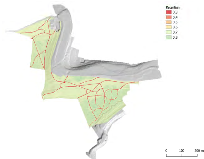
Figure 10. Potential retention of rainwater at the site expressed by the retention coefficient—modelled state after site destruction (prepared by authors).
