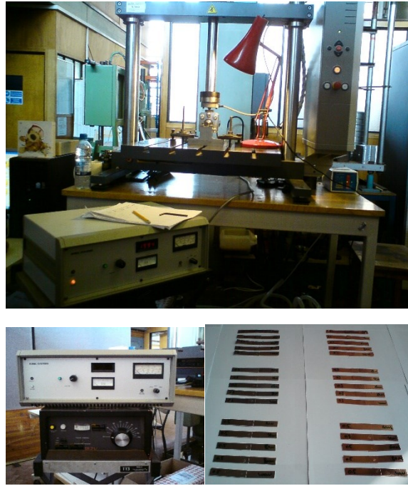
Fig. 2. Setup of ultrasonic welding device and their accessories with generator, controller and sets of spot welded specimens
