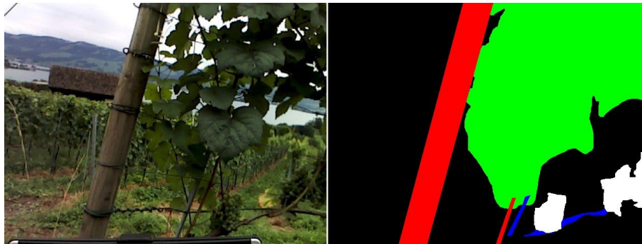
Figure 2.2. An example of (image-mask) tuple used for semantic segmentation.
