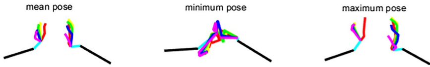
Fig. 4 Discriminative poses consist of mean pose, the average of all hand poses in the sequence; minimum pose where hands are closest together; and maximum pose where hands are furthest apart
