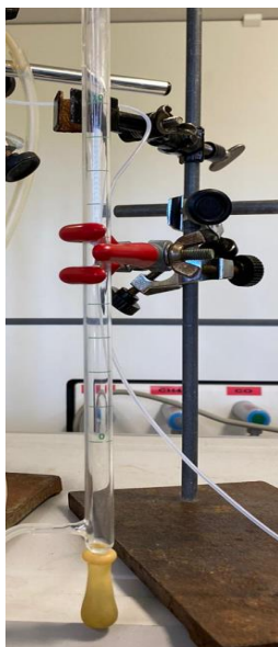
Figure 3.9. Manual soap bubble flow meter.
