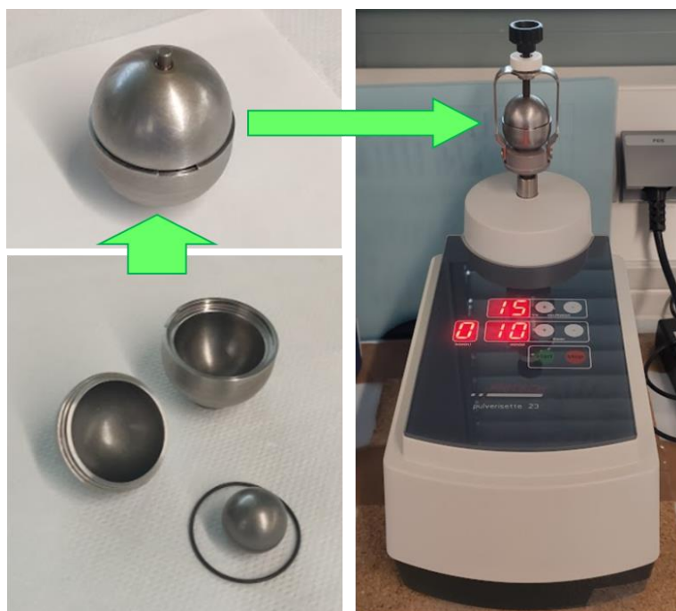
Figure 3.8. Ball mill equipment and used grinding ball and bowl.
