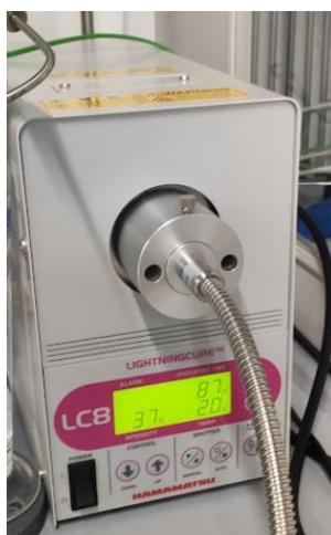
Figure 3.5. Light source LC8 from HAMAMATSU.
