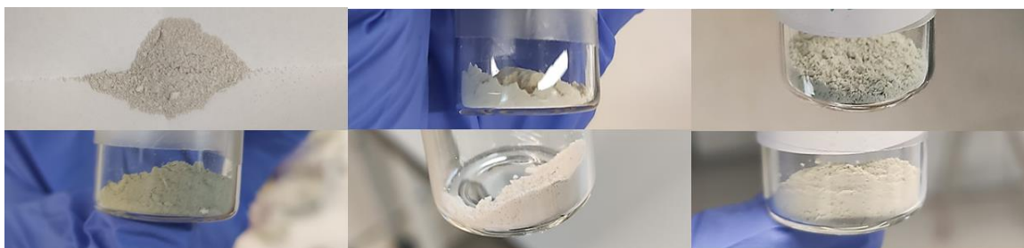
Figure 4.5. From left to right, fresh (above) and 2 nd (below) TiO 2 /PdPtMe powders with Au, Ag and Cu.
