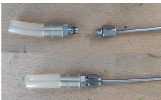
Figure 3.7. Fabricated tubing and connections (upper components: detached Swagelok® connection; and lower components: plugged gastight Swagelok® connection).
