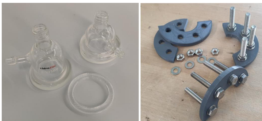
Figure 3.4. Reactor halves, PDMS O-ring and some of the used 3D printed pieces.
