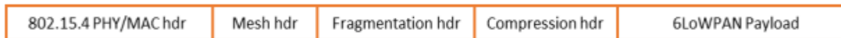
Figure 2.12: 6LoWPAN Packet Containing Mesh Hader for Layer 2 Forwarding, a Fragmentation Header and a Compression Header
