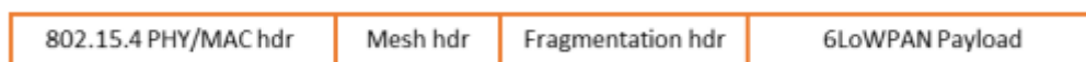
Figure 2.13: 6LoWPAN Packet Representing Subsequent Fragments that Do Not Contain Any Information about the IPv6 Header
