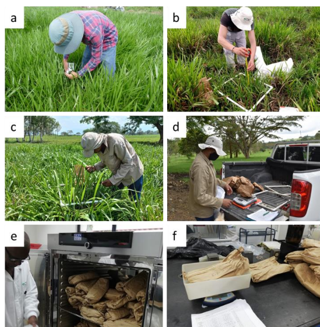
Figure 2. Image examples of manual measurements and sample collection in the field. (a) SPAD values measured in the plot G10; (b) height measurement collected in the plot G03; (c) forage fresh matter production measures in the plot G10; (d) weighing fresh matter; (e) oven drying of samples; and (f) weighing dry matter.
