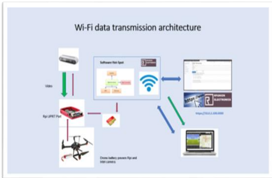
Fig. 4.8 Wi-Fi architecture @ Francesc Capdevila. In this image we can see how the different systems interact, on the right side of the image we have the base station (laptop) which via Wi-Fi is connected to the hot spot of the drone and in turn connected to the rpanion website , where we can change the parameters. In the center of the image we have the SD card, on it we find the rpanion software
