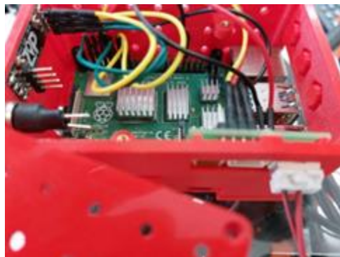
Fig. 4.2 Wiring necessary to light up the LED's. CTTC Castelldefels, Francesc Capdevila (03-2022) The wires on the left are the ones that connect the LED lights to the Raspberry pins and the UART port.
