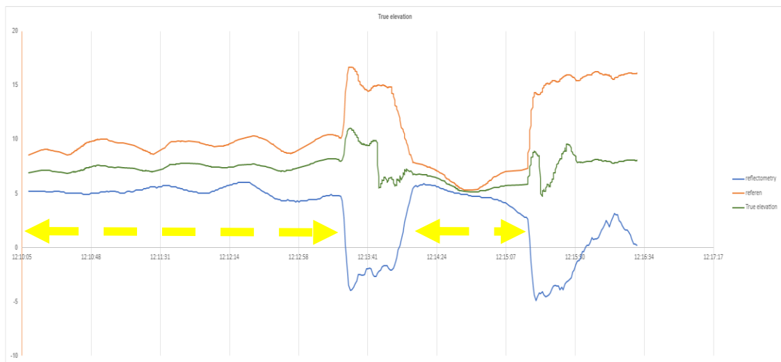
Fig. 5.13 True altitude after comparing both data (green line). The orange line indicates the altitude from the drone antenna, the blue line indicates the altitude from the reflectometry antenna, and the green line shows the true altitude of the drone in the dronelab. The yellow dotted line shows the drone in stationary flight. The vertical axis is the altitude in meters and the horizontal axis is the last five minutes of flight in seconds.
