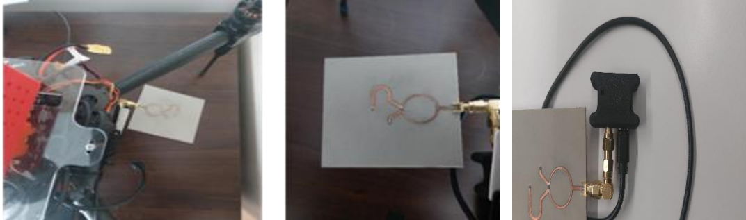
Fig. 1.1 GNSS antenna made by Pedro Espin and Fermín Mira at CTTC for the project. Francesc Capdevila CTTC (03-2022). The left and center photos are the reflectometry antenna, the right photo is the receiver.
