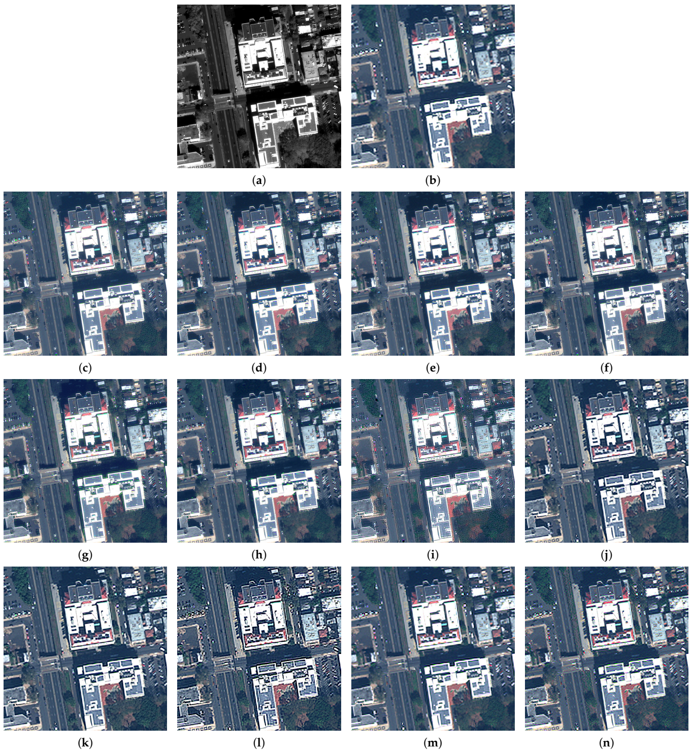
Figure 4. Fusion results at full resolution, using a true-color representation, for the Trenton dataset: (a) Pan image; (b) expanded; (c) GS; (d) BT; (e) HCS; (f) GSA; (g) BT-H; (h) HECS; (i) BDSD; (j) AWLP-H; (k) MTF-GLP-FS; (l) SR-D; (m) TV; (n) A-PNN-FT.
