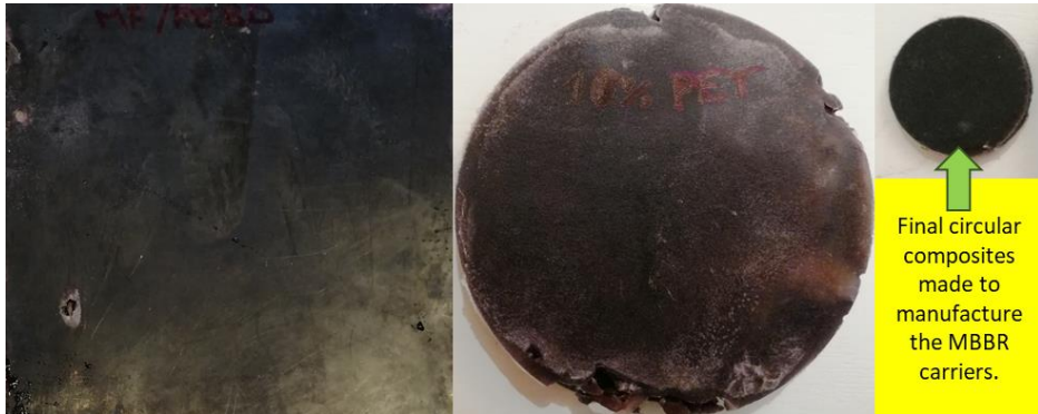
Figure 10.3. Plates formed with the pressuring machine. The final circular composites were obtained from the squared composites.
