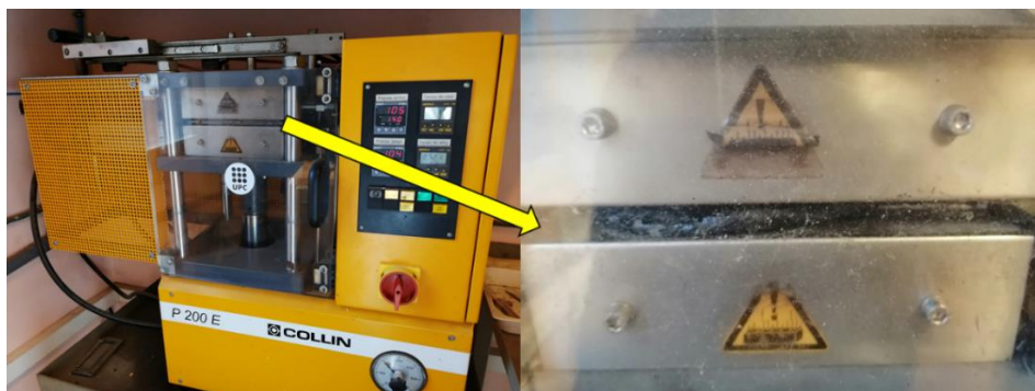
Figure 10.2. The composite is being compressed by the pressuring machine.
