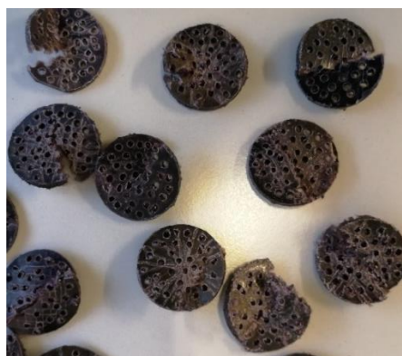
Figure 10.4. MBBR carriers with holes to increase the specific area and give supporting places for the microorganisms to attach.
