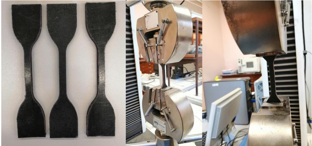
Figure 10.5. Tensile test machine used to test the composites. The image from the left corresponds to the test pieces formed to make the testing experiment according to the ASTM-D-638-14.
