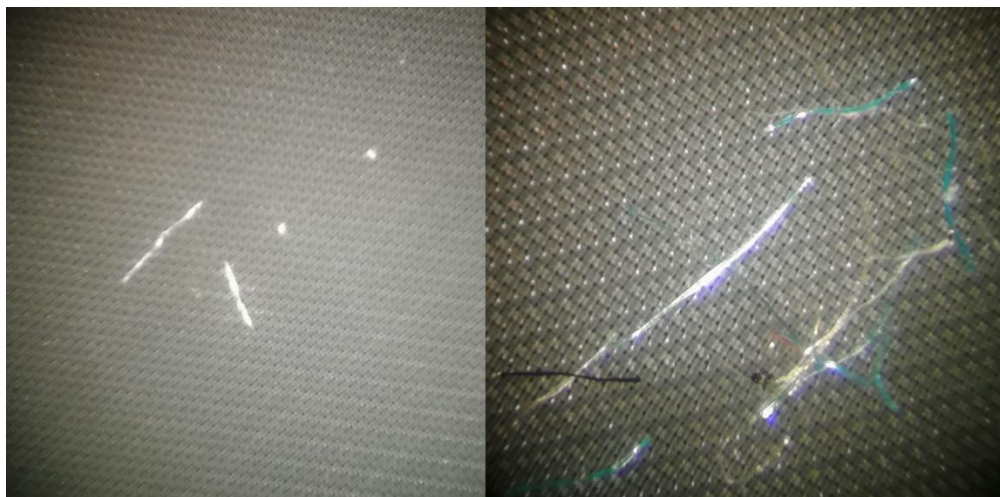
Figure 1.9. Textile microfibers retained by filtering a laundering effluent.
