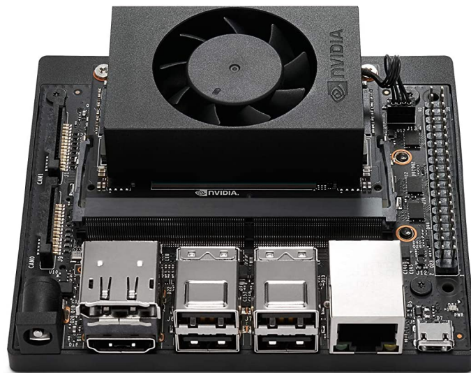
Figure 3.1: The Jetson Xavier NX developer kit [6].
