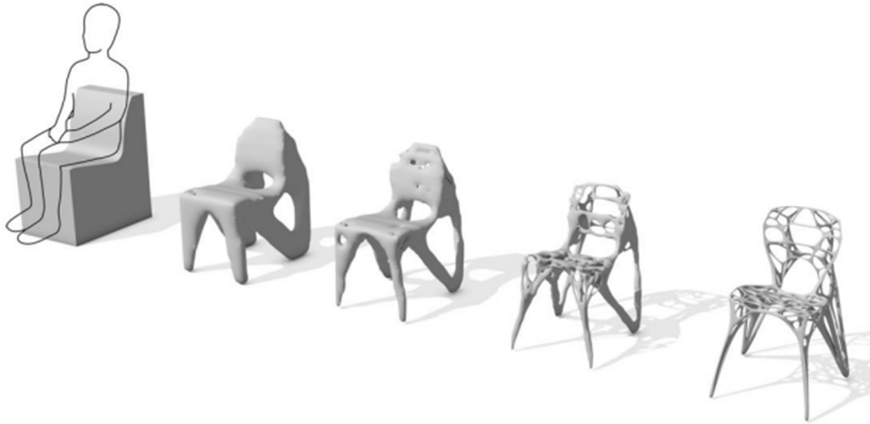
Figure 2.13 3-D printed Topology Optimized chair
