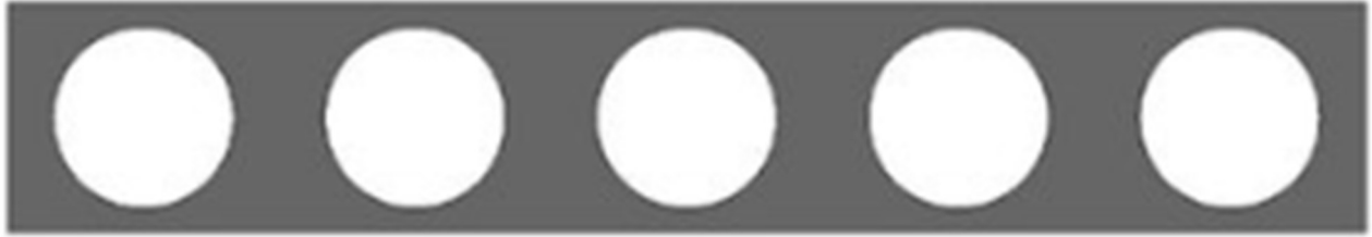
Figure 2.7 Shape Optimization problem Given Load assignments, restraint assignments, topology and initial external and internal boundaries (Geometry)
