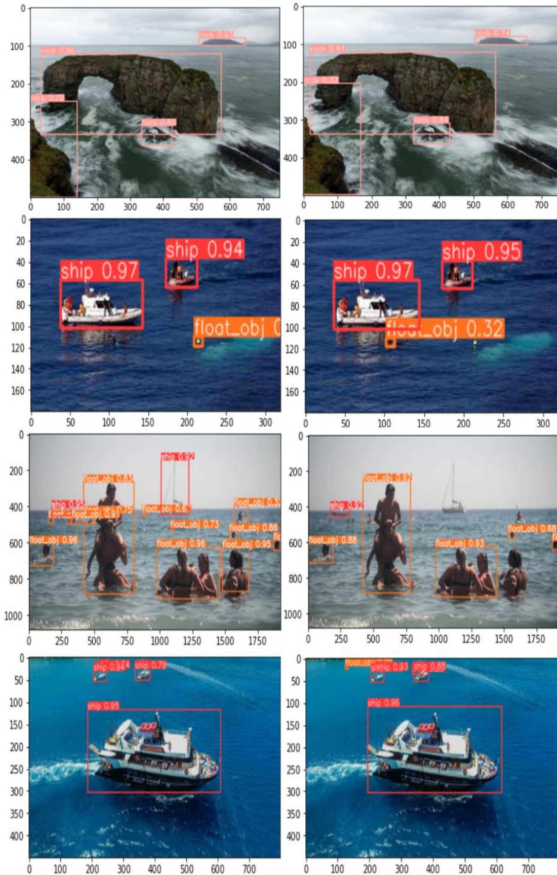
Figure 4.16: Comparison between YOLOv5s and YOLOv5m trained on the same 400 images for 300 epochs and batch size of 8. The right images are the results from the YOLOv5s model and the left are from YOLOv5m
