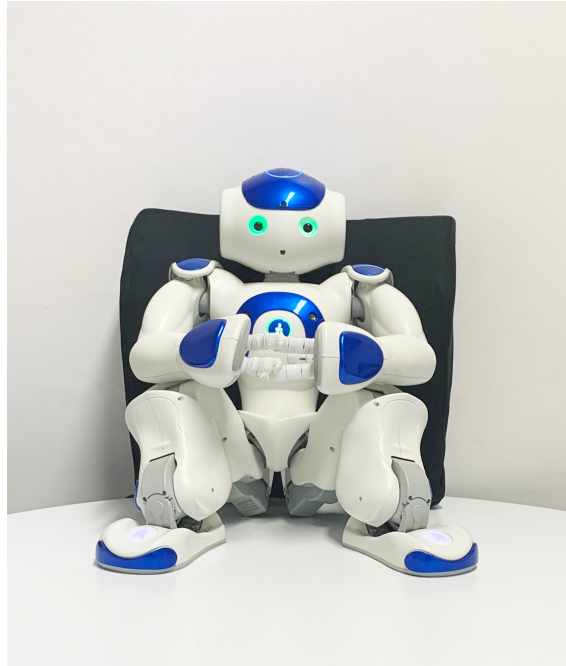
Figure 3.1: The robot used in Study 2: A NAO V5 by SoftBank Robotics
