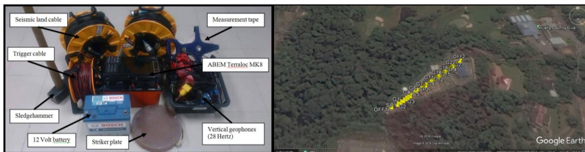
Figure 2. Seismic refraction equipment set.
