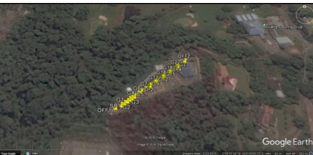
Figure 3. Spread line performed at site studied.
