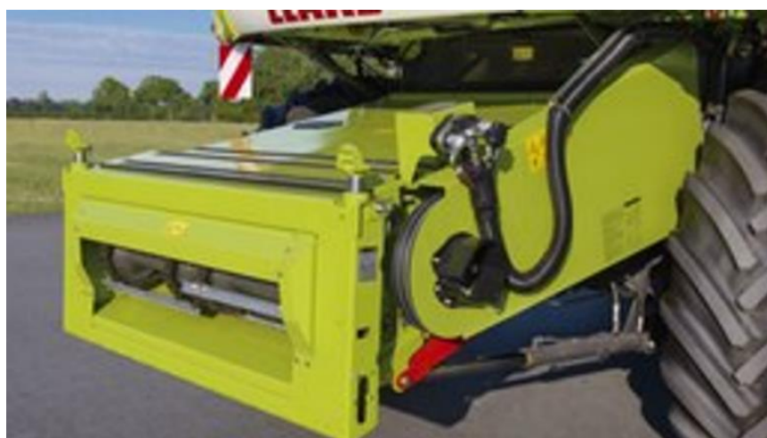
Fig. 3.9. CLAAS combine harvester feeding house
