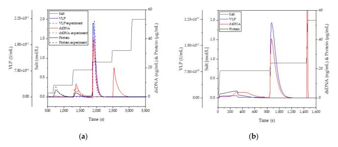
**Figure 10.** Results of the parameter determination (**a**). Dashed lines are the experimental results; solid lines are the digital twin results. In (**b**), the results for a potential optimized and scaled-up capture step are given.
