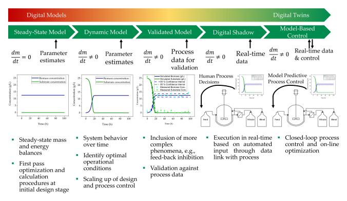
**Figure 1.** Levels of a digital twin, starting from a steady-state model to a dynamic model, a validated model, and a digital shadow to a model-based control.
