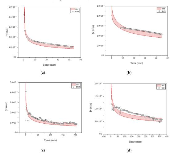
**Figure 9.** Flux Jv over time for experimental (squares) as well as digital twin prediction (red area) for ultrafiltration/diafiltration experiments and concentration factor 7. (**a**) Experiment 1 (EXP1): 1.5 bar transmembrane pressure (TMP), 3738 s<sup>-1</sup> shear rate. (**b**) Experiment 5 (EXP5): 0.5 bar TMP, 3738 s<sup>-1</sup> shear rate. (**c**) Experiment 6 (EXP6): 0.5 bar TMP, 1249 s<sup>-1</sup> shear rate. (**d**) Experiment 8 (EXP8): 1.5 bar TMP, 1249 s<sup>-1</sup> shear rate.
