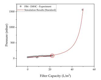
**Figure 7.** Data points used for the regression to determine the blocking constant and the modeling via the standard blocking model resulting from the parameter determination.
