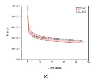
**Figure 8.** Flux Jv over time for experimental (squares) as well as digital twin prediction (red area) for ultrafiltration/diafiltration experiments and concentration factor 3. (a) Experiment 2 (EXP2): 1.5 bar transmembrane pressure (TMP), 3738 s<sup>-1</sup> shear rate. (b) Experiment 3 (EXP3): 1.5 bar TMP, 1249 s<sup>-1</sup> shear rate. (c) Experiment7 (EXP7): 0.5 bar TMP, 3738 s<sup>-1</sup> shear rate.
