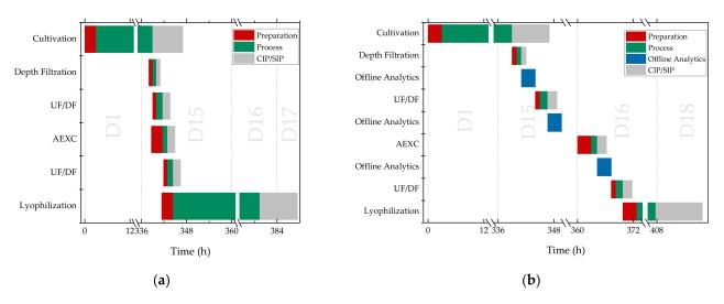
**Figure 13.** Optimized process schedule enabled by PAT for APC and DT (**a**) vs. conventional process schedule based on offline analytics (**b**).
