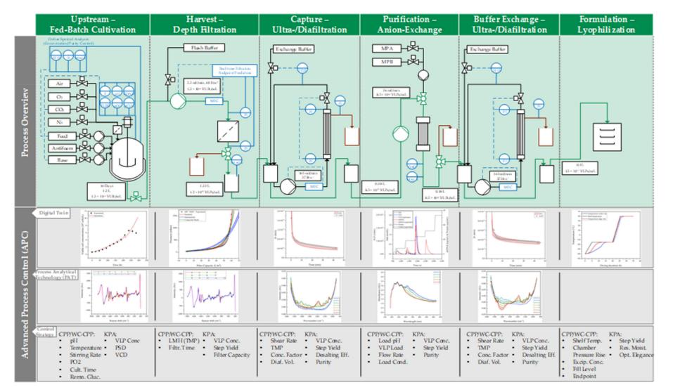
**Figure 12.** Process flowsheet including APC by digital twins and optimized PAT. Critical Process Parameter (CPP), Well-Controlled Critical Process Parameter (WC-CPP), Key Process Attribute (KPA), particle size distribution (PSD), Viable Cell Density (VCD), transmembrane pressure (TMP), virus-like particle (VLP).
