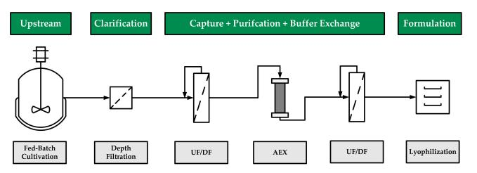
**Figure 3.** Process flow diagram showing the production and subsequent three-step purification of HIV-gag VLPs. Capture is achieved by depth filtration, ultrafiltration/diafiltration (UF/DF) is used for concentration and initial purification, anion exchange chromatography is used for further purification and concentration, and lyophilization is used for the formulation of HIV-gag VLPs.
