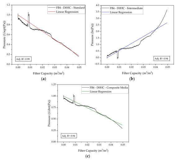
**Figure 5.** Characterization of blocking mechanism during constant flux direct (not pre-clarified) depth filtration of FB4 (Millistak<sup>®</sup> + D0HC) by linear regression. Regression results of standard (**a**), intermediate (**b**), and composite media models (**c**). Black squares represent the experimental pressure values.
