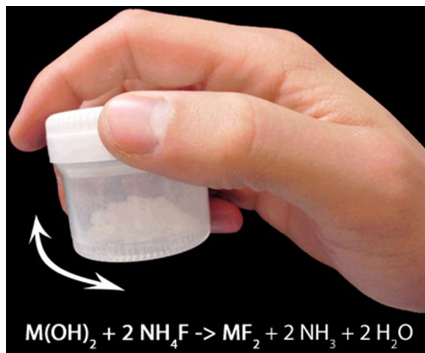
Fig. 6 Illustration of the preparation of alkaline earth metal fluorides \text{MF}_2 , simply by shaking. Reproduced from [67]. Copyright 2012 Elsevier Masson SAS. All rights reserved
