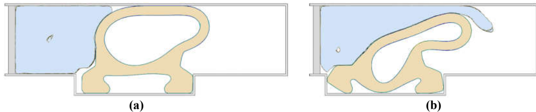
Fig. 3.31: 1° segment of the axisymmetric seal studied by Morrison et al. 215 (a) with a pressurised fluid prior to leakage; (b) as fluid breaches the sealing interface. (Images adapted from Gorash.) 219
