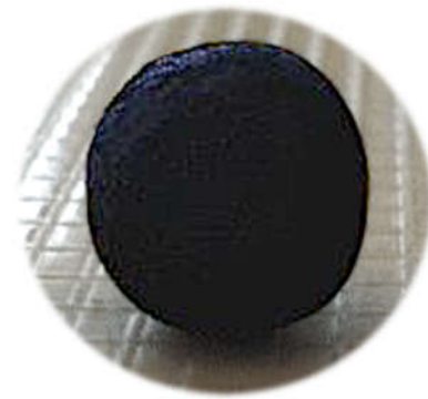
Fig. 2.35: Carbon black mixed with low viscosity paraffin oil. (Adapted from Warasitthinon et al. ) 132
