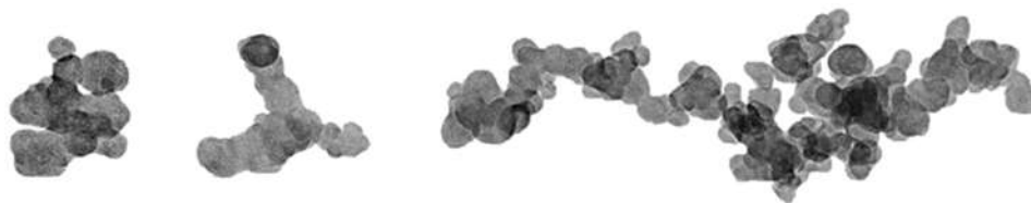
Fig. 2.41: Carbon black aggregates with structure increasing from left to right. (Adapted from Hallet & Tunnicliffe.) 139
