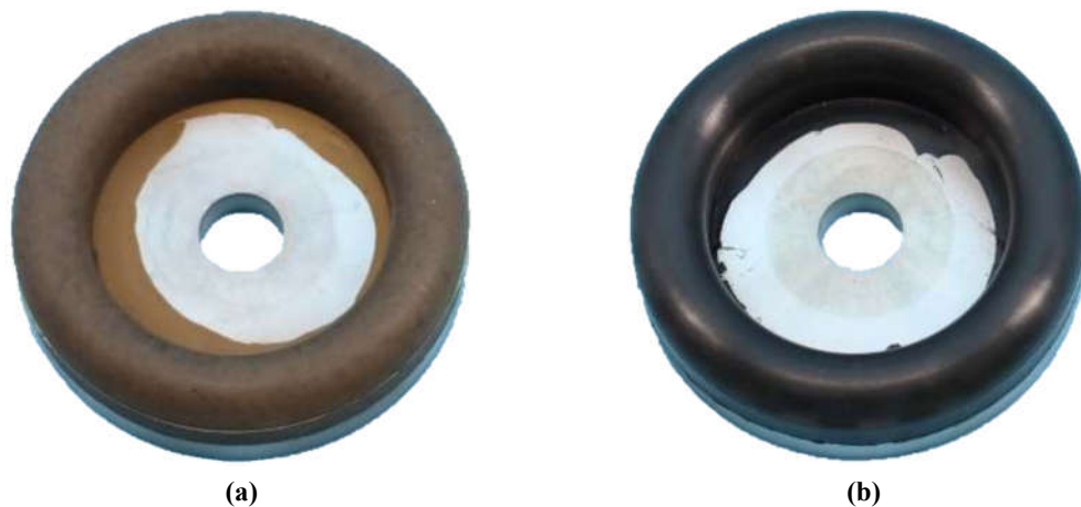
Fig. 6.5: Bonded rubber seals: (a) the unfilled natural rubber; (b) the silica-filled EPDM rubber.
