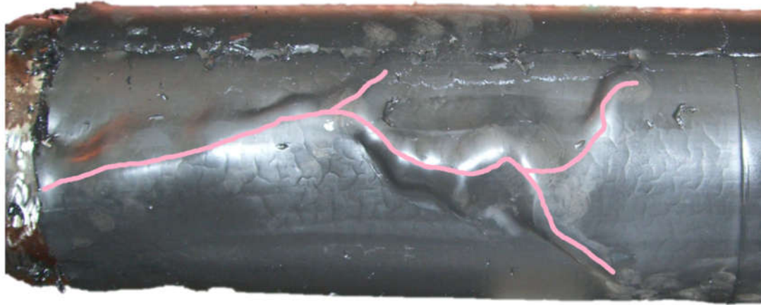
Fig. 8.1: Evidence of fluid penetration along the inner diameter of a swell packer. The leak paths are indicated by the pink curves. (Adapted from Eatwell.) 268
