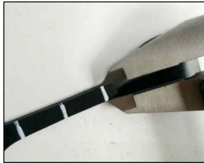
Fig. M.1: Measurement of the dumbbell width with the tip of the calipers positioned at the top face of the specimen. The bottom face would also be measured. Multiple positions along the length, for instance 6 total places, can be measured and averaged.
