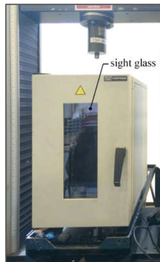
Fig. 4.9: Thermal test chamber with sight glass.
