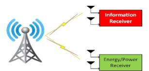
Figure 2 Simultaneous information and power transfer
