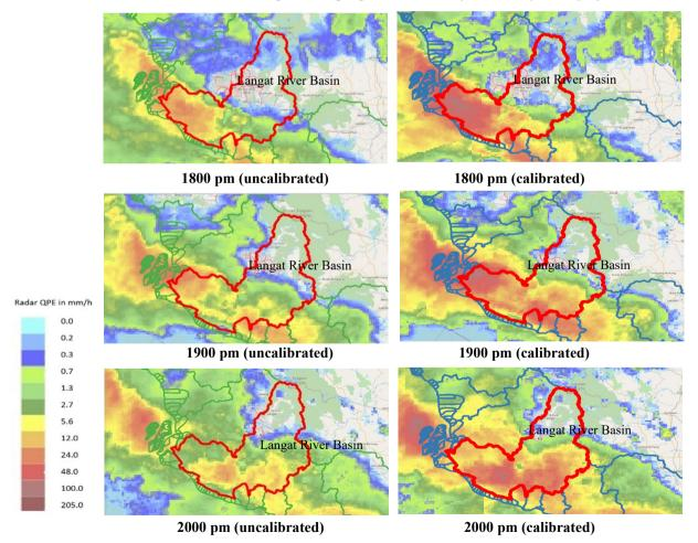
Fig. 8 - Comparison between uncalibrated radar QPE and calibrated radar for Langat River Basin during flood event on 17<sup>th</sup> December 2021
