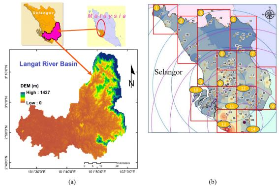
Fig. 6 - (a) Map showing the location of Selangor and Langat River Basin, Selangor, Malaysia [24]; and (b) radar coverage from KLIA and Subang radar and zoning of smaller region for MFB based on rainfall gauge cluster over isopleth of median ratio
