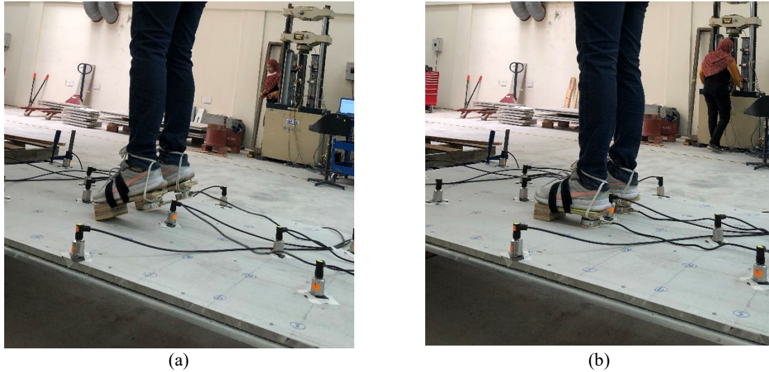
Fig. 8 - Heel-drop test position (a) rises toes; (b) sudden drop
