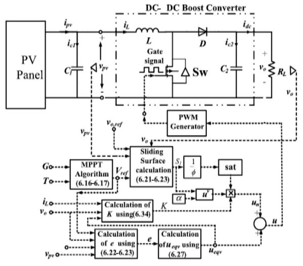
Fig. 3 SISMC based MPPT design
