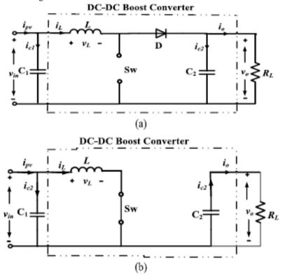
Fig. 2 DC-to-DC Boost converter operation (a) when switch is open u=1; (b) when switch is closed u=0
