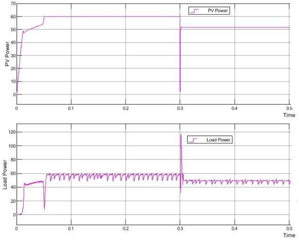
Fig. 5 - Load and source output power variation of SISMC design
