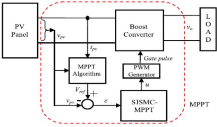
Fig. 1 Schematic view of solar PV system model with SISMC
