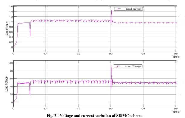
Moreover, it is measured that the sliding surface duty cycle ratio of the sliding mode MPPT control scheme is at 0.7226 only. Therefore, the sliding duty cycle ratio of SMC scheme is limited to effective dynamic sliding surface switching operation compared to the present SISMC MMPT scheme. This authenticates that, the proposed SISMC
