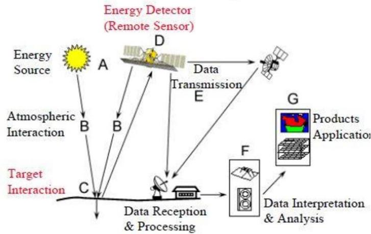
Fig. 4 - Remote sensing process [26]
