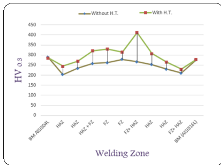
Fig. 7 - Micro hardness values of the optimum stud welding specimen with and without PWHT
