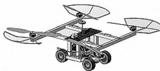
Figure 16. Ground and air dual-use information gathering robot
